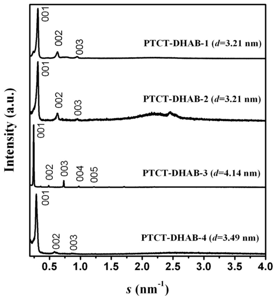
Fig. S9 X-ray diffraction patterns of PTCT-DHAB-1, PTCT-DHAB-2, PTCT-DHAB-3 and PTCT-DHAB-4. (Miller indices are used to assign the reflections; the traces are offset for clarity).
