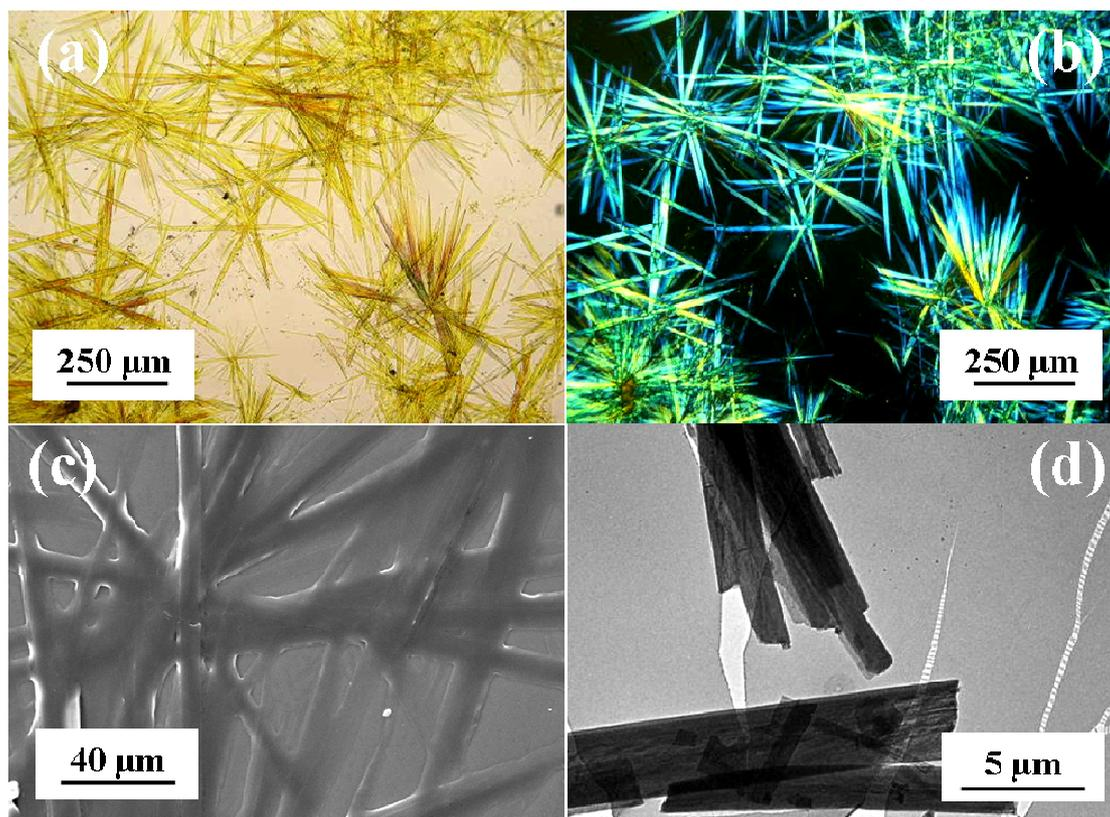
Fig. S8 Morphology of PTCT-DHAB-3 precipitated from toluene solution with acetone: (a) POM image, (b) POM image under crossed polarizers, (c) SEM image and (d) TEM image.
