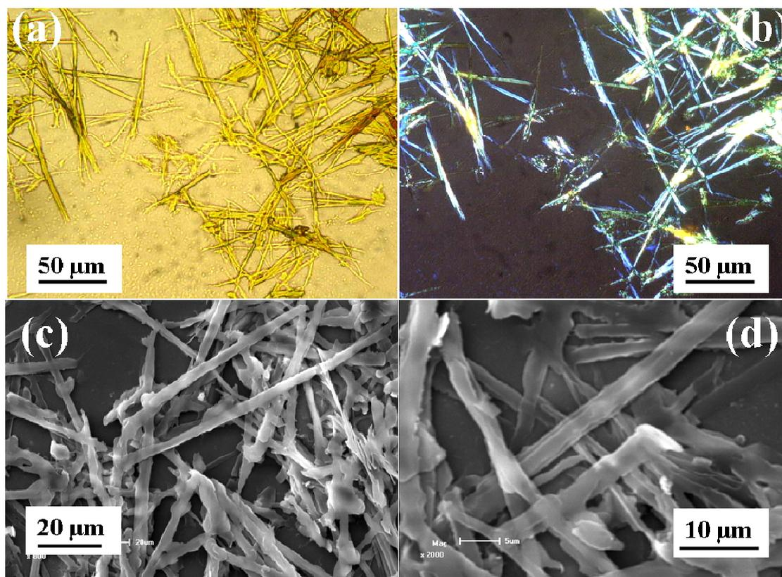
Fig. S7 Morphology of PTCT-DHAB-2 precipitated from ethanol solution with water: (a) POM image, (b) POM image under crossed polarizers, (c) and (d) SEM images.
