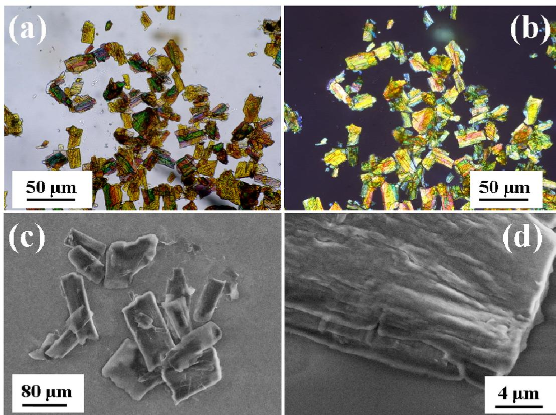
Fig. S6 Morphology of as-prepared PTCT-DHAB-1: (a) POM image, (b) POM image under crossed polarizers, (c) SEM image and (d) higher-magnification SEM image over an aggregate.
