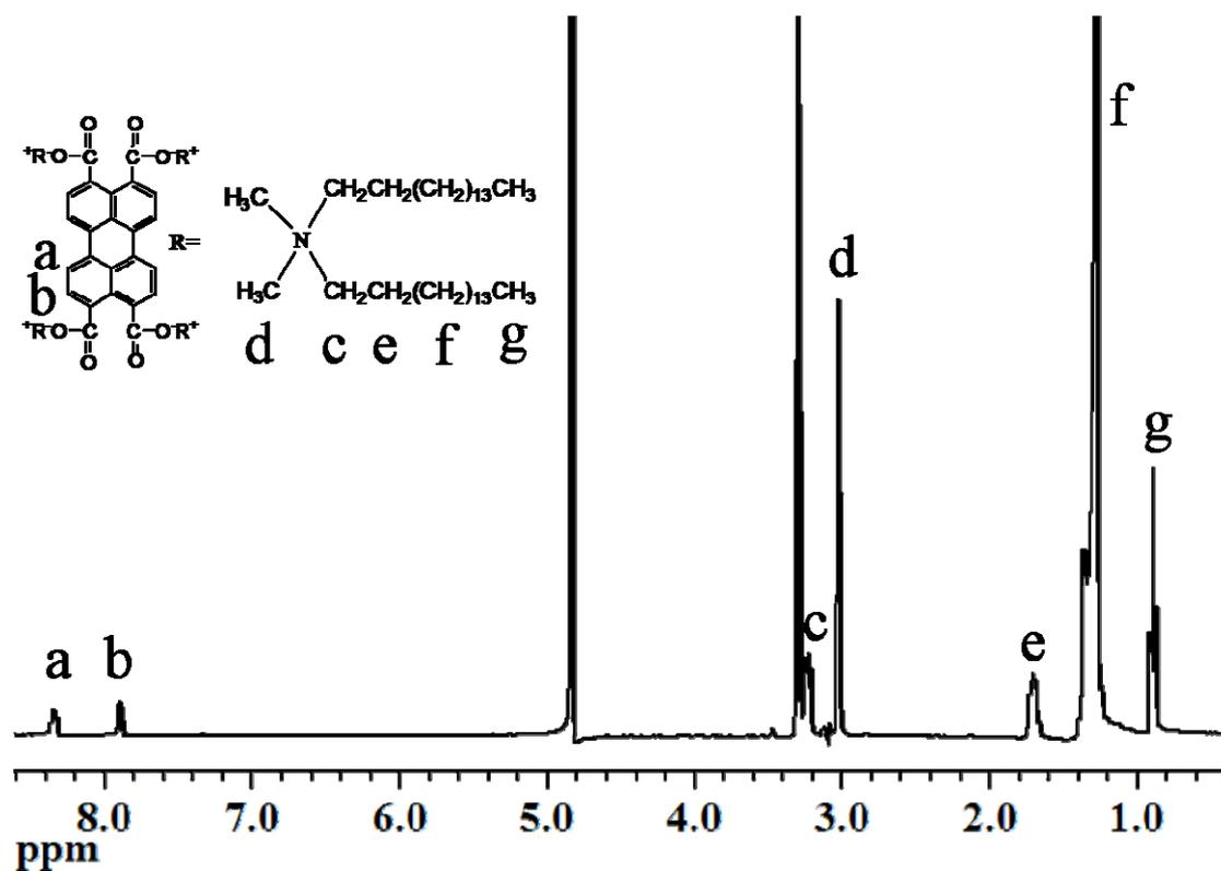
Fig. S3 <sup>1</sup>H-NMR spectra of PTCT-DHAB.
