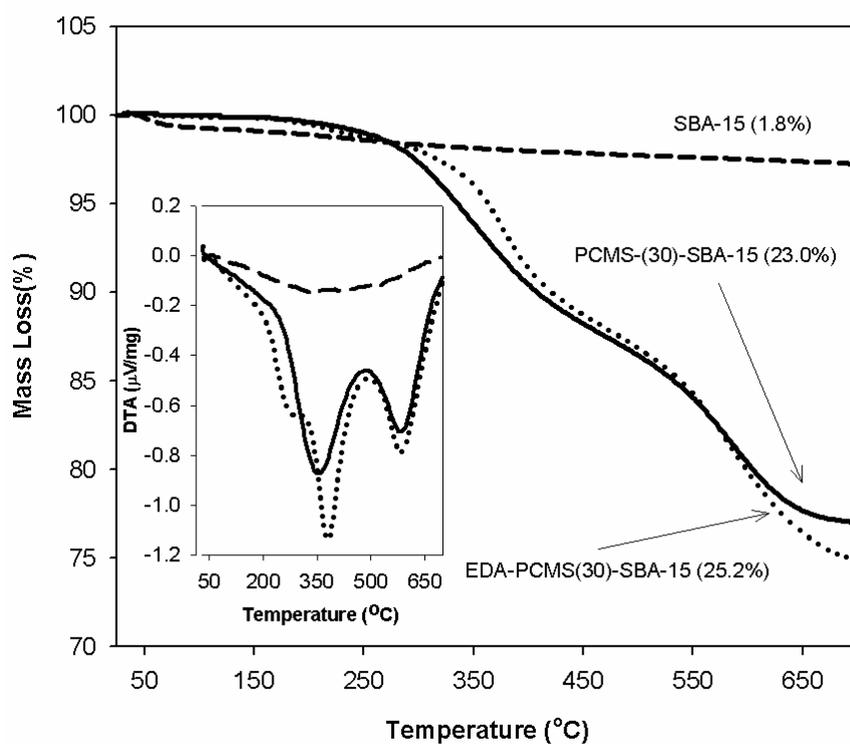
**Figure S2** TGA curves of the PCMS(30)-SBA-15 composite before and after treatment with EDA. Inset: DTA analysis (pure SBA-15 is shown as a reference).
