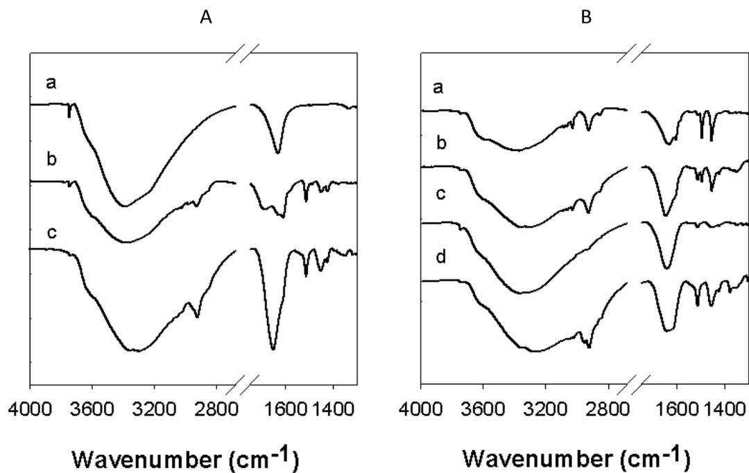
**Figure S3** ATR-FTIR spectra of A: a) KIT-6; b) PCMS(30)-KIT-6; and c) EDA-PCMS(30)-KIT-6, and B) a) EDA-PCMS(0.1; 30)-SBA-15; b) EDA-PCMS(0.5; 30)-SBA-15; c) EDA-PCMS(10)-SBA-15 and d) EDA-PCMS(30)-SBA-15.
