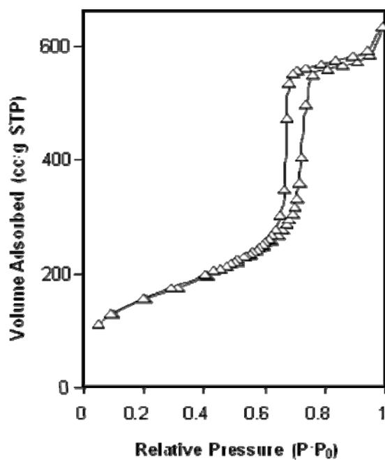
**Figure S1** N<sub>2</sub> physisorption isotherm of EDA-PCMS(30)-KIT-6 measured at -196 °C.
