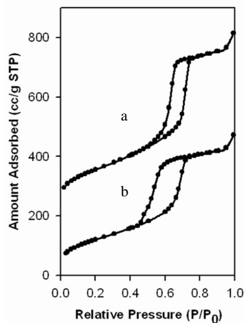
**Figure S4** N<sub>2</sub> sorption isotherms of EDA-PCMS:PS composites, a) PCMS(0.1; 30)-SBA-15 (offset is 250 cm<sup>3</sup>g<sup>-1</sup>); b) PCMS(0.5; 30)-SBA-15.
