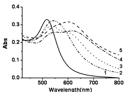
**Figure S4.** UV-vis spectra of gold nanoparticles with “trimethyl lock” peptide substrate (8.5  $\mu\text{M}$ ) treated with esterase (12.5  $\mu\text{g/mL}$ ) as a function of time. The time interval is 0.5 hr from state 1 to state 5.
