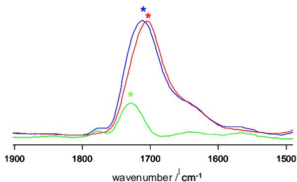
**Figure S1. Model reaction between maltose and PEMA in thicker films to exhibit ester bond formation.** ATR-IR spectra of mixture between maltose and PEMA as film on Si wafer. Molar ratio between maltose and PEMA is 2. Red IR spectrum belongs to mixture of maltose and PEMA which was dried at room temperature. Blue IR spectrum belongs to mixture of maltose and PEMA which was annealed at 120°C for 2h. Green IR spectrum belongs to the subtraction of red spectrum from blue spectrum.
