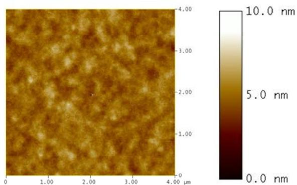
**Figure S5.** AFM height images of dry PEI-Mal film ( $d = 100$  nm) after annealing and washing/drying step (after step (ii) in Scheme 1); PEI-Mal film cross-linked with PEMA hydrolyzed.
