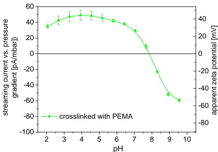
**Figure S4.** pH dependence of the streaming current versus pressure gradient and apparent zeta potential for PEI-Mal film with cross-linker poly(ethene-*alt*-maleic anhydride) (PEMA) (film thickness 110 nm) at 1 mM KCl solution. The measurements were performed at a channel height of 30  $\mu\text{m}$ . Explanation for apparent zeta potential is presented in the method section in ESI.
