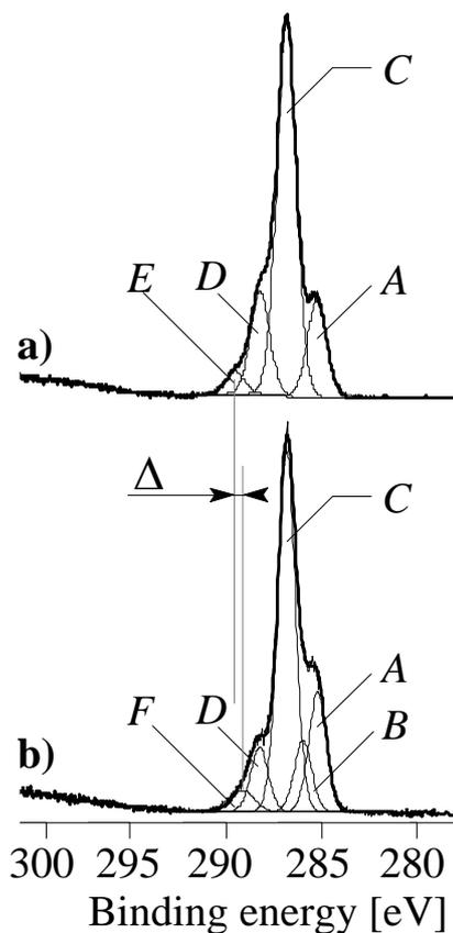
**Figure S2.** High-resolution C 1s X-ray photoelectron spectra of a maltose reference sample (a) and maltose reacted with PEI and subsequently cross-linked with hydrolyzed poly(ethylene-*alt*-maleic anhydride) (b). The difference between component peak *F* and component peak *E* ( $\Delta$ ) illustrates the presence of carbonic ester groups.
