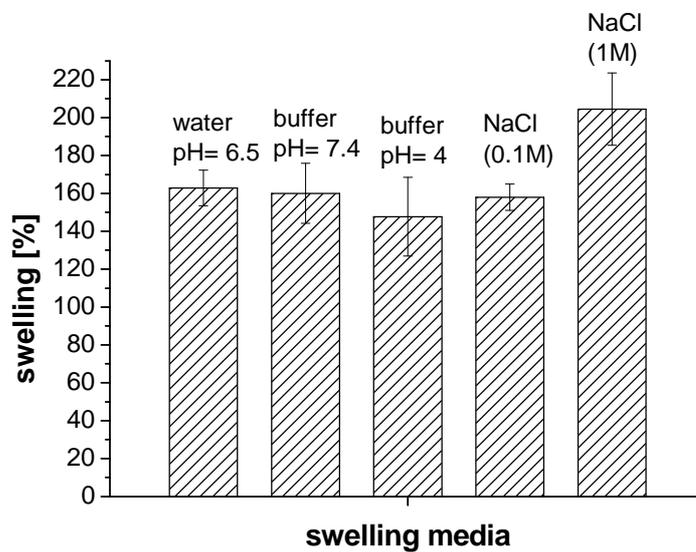
**Figure S7.** Swelling behavior of thin PEI-Mal film series cross-linked with PEMA deposited in different media.
