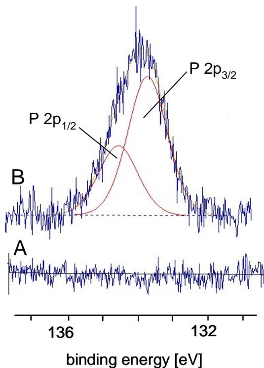
**Figure S9.** High-resolution P 2p X-ray photoelectron spectrum of PEI-Mal film (cross-linked with PEMA) with  $d = 100$  nm showing the phosphorus atoms on the topmost surface of dried PEI-Mal film (A) before ATP adsorption and (B) after the ATP adsorption followed by two rinsing steps with water.
