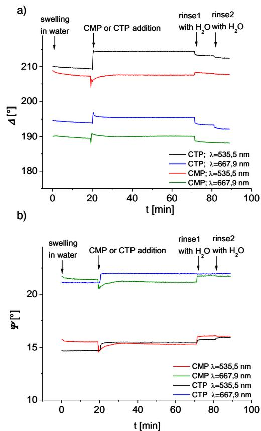
**Figure S8.** Dynamic scan of the experimental ellipsometric scan of the parameters  $\Delta$  (a) and  $\Psi$  (b) (e.g. for  $\lambda = 535.5$  and  $667.9$  nm) during the swelling in water, addition of CTP and CMP (both:  $c = 0.5$  mg/ml) and rinsing process with water of PEI-Mal films cross-linked with PEMA.
