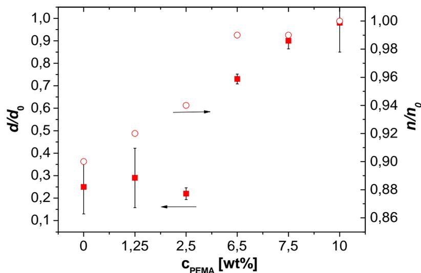
**Figure S3.** Stability of dry PEI-Mal films in dependence of the cross-linker concentration for poly(ethene-*alt*-maleic anhydride) (PEMA) hydrolyzed.
