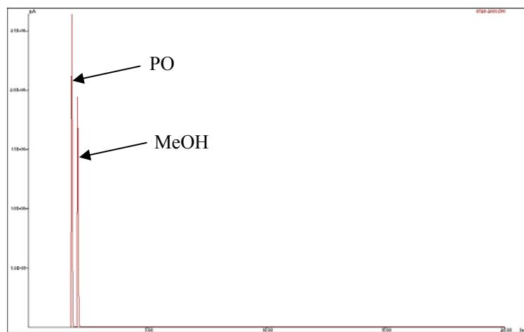
b) GC trace for the mixture after reacting PO and MeOH catalyzed by [TMG][Ac]
