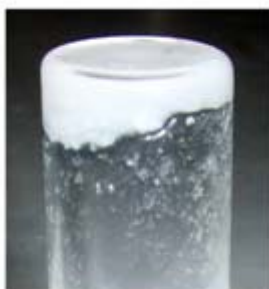
Figure S1. Photographs of a gel of 3 in an inverted glass tube.
