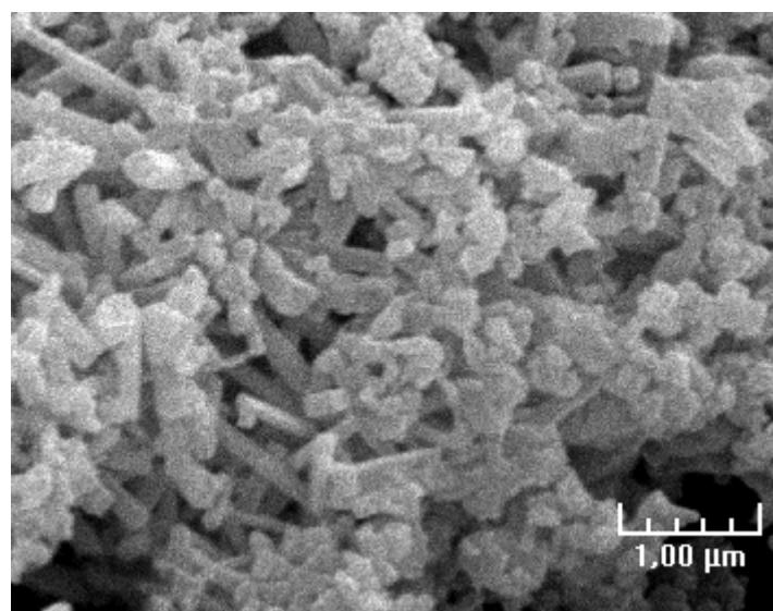
Figure S2. SEM photograph of DMOF-NH<sub>2</sub> (1)
