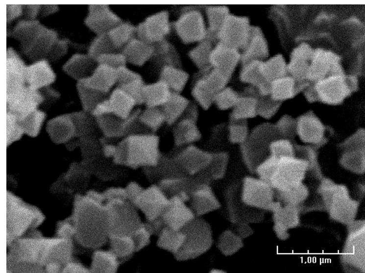
Figure S10. SEM photograph of MIL-101(Fe)-NH<sub>2</sub> (5)
