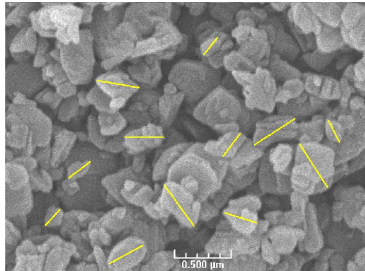
**Figure S8. : SEM photograph of MIL-53(Al)-NH<sub>2</sub> (4)**
