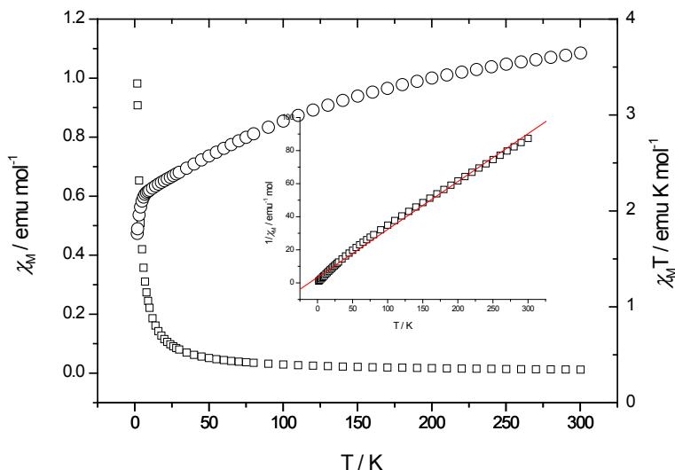
Fig. 3S Plots of molar magnetic susceptibility  $\chi_M$  (□, left) and  $\chi_M T$  (○, right) vs.  $T$  for compound **5**. Inset: Reciprocal dependence of the magnetic susceptibility on temperature. The solid lines result from least-square fits of the Curie-Weiss Law. The fitting results are  $g = 2.146$ ,  $\theta = -11.59$  K.
