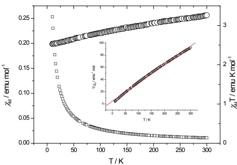
Fig. 2S Plots of molar magnetic susceptibility  $\chi_M$  (□, left) and  $\chi_M T$  (○, right) vs.  $T$  for compound **3**. Inset: Reciprocal dependence of the magnetic susceptibility on temperature. The solid lines result from least-square fits of the Curie-Weiss Law. The fitting results are  $g = 2.104$ ,  $\theta = -14.328$  K.
