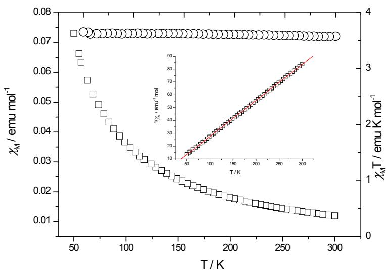
Fig. 1S Plots of molar magnetic susceptibility  $\chi_M$  (□, left) and  $\chi_M T$  (○, right) vs.  $T$  for compound **1**. Inset: Reciprocal dependence of the magnetic susceptibility on temperature. The solid lines result from least-square fits of the Curie-Weiss Law. The fitting results are  $g = 2.179$ ,  $\theta = 2.054$  K.
