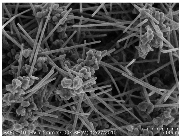
Figure 5. SEM image of general view of Cu@C nanowires prepared at 150°C for 15 h.
