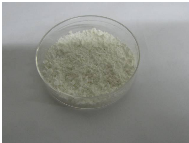
Figure S1. Photo of powder of \text{Gd}(\text{OH})_3 nanorods. The sample was totally dried and placed in one 4cm dish. The nanorods 5 were synthesized in two Teflon-lined stainless-steel autoclaves (50 mL).
