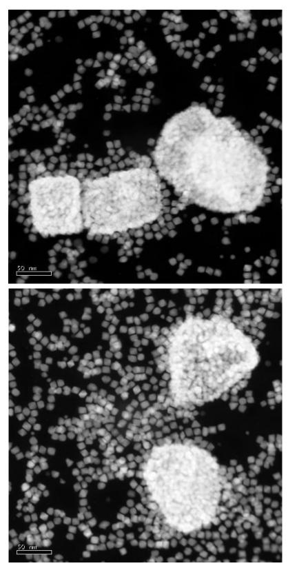
Self-assembly of Pt nanoparticles is discovered. Novel Pt nanotextures show evidences originating from surface-attachment, self-aggregation, self-agglomeration and self-assembly through novel discoveries of surface attachments.
