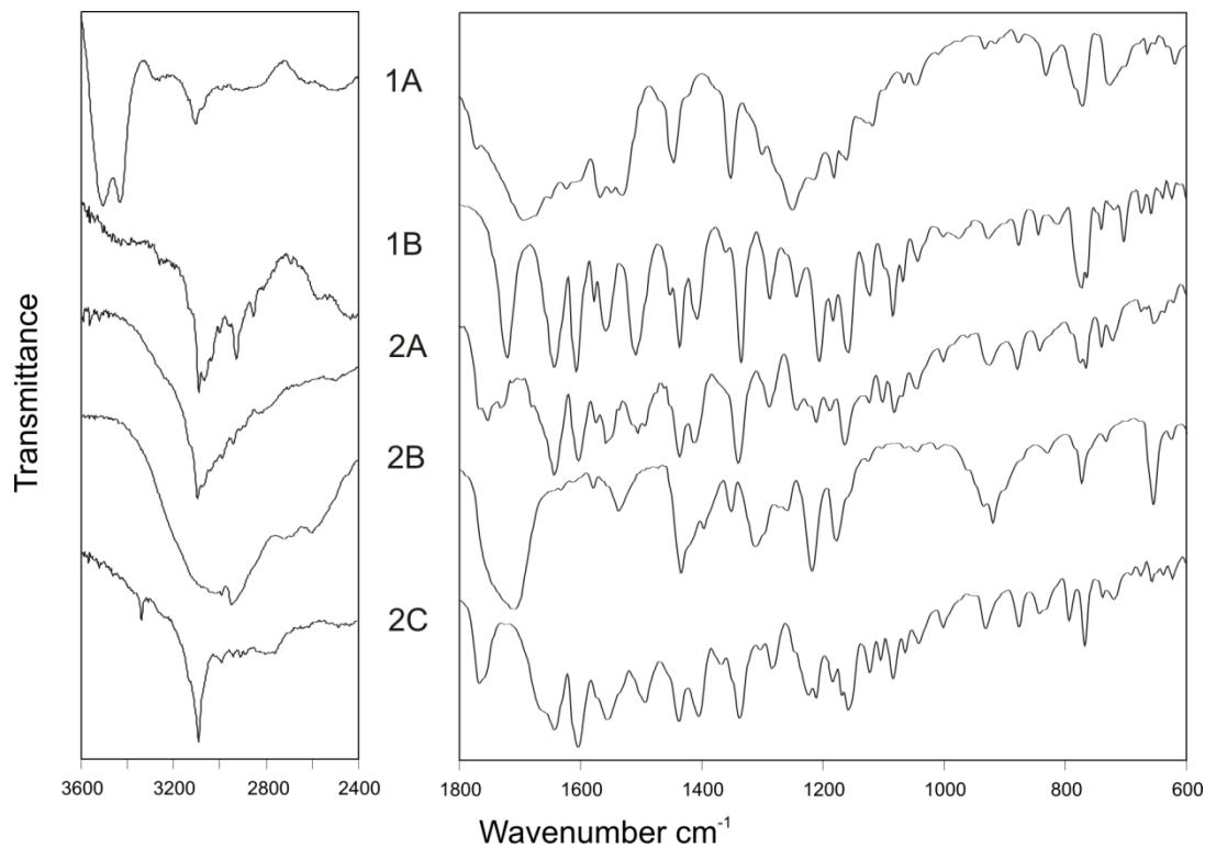
**Fig. S 2** IR spectra of the co-crystals with oxalic acid and malonic acid as guest.
