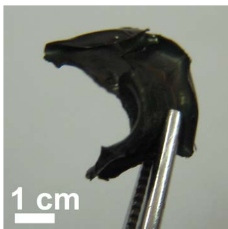
Fig. S2. Digital photo of dried \alpha -Fe 2 O 3 /graphene composite at 80°C for 24h.
