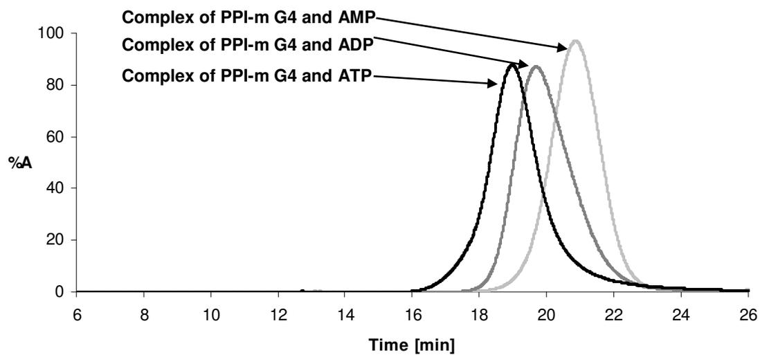
**Fig.1.** Chromatograms of separating of complexes PPI-m G4 dendrimer with ATP, ADP and AMP. (20 mmol/L HEPES buffer with 150 mmol/L NaCl, pH 7).
