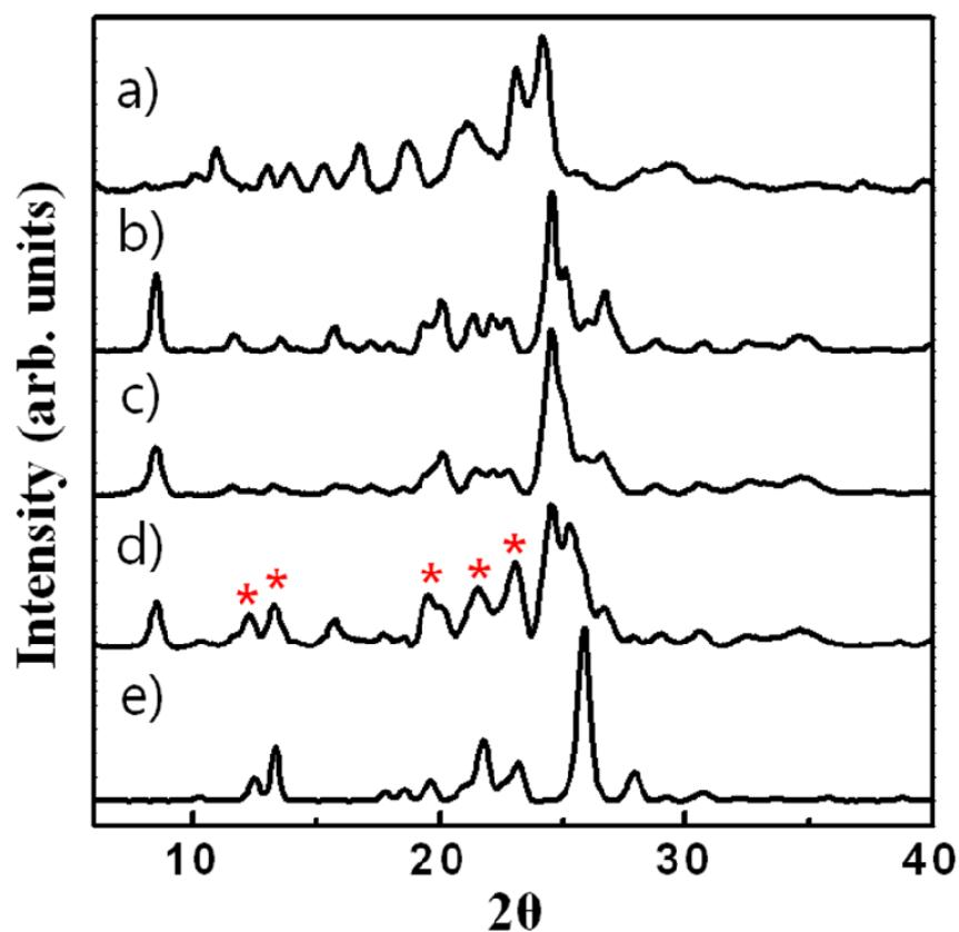
**Fig. S4** Powder X-ray diffraction pattern of (a) xerogel **1** with 1.0 equiv of **2** and (b) crystal **1** obtained from 2.0 equivalent of **2**, xerogel **1** with (c) 2.0 and (d) 3.0 equiv of **2**, and (e) free **2** (4,4-bipyridine):
