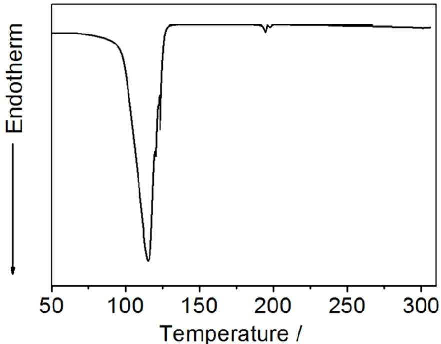
**Fig. S5** DSC thermogram of gel **1** with 1.0 equivalent of **2**.
