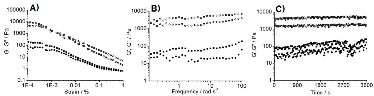
**Figure S6.** Dynamic oscillatory and steady shear measurements of gel **1** at different concentration of **2** at 25 °C: A) strain sweep at a frequency of 1 rad s<sup>-1</sup>; B) frequency sweep at a strain of 0.01%; C) time sweep at a strain of 0.01% and frequency of 1 rad s<sup>-1</sup>; **1**: **2**=1:1 ■:  $G'$ , ●:  $G''$ ; **1**: **2**=1:3 □:  $G'$ , ○:  $G''$ .
