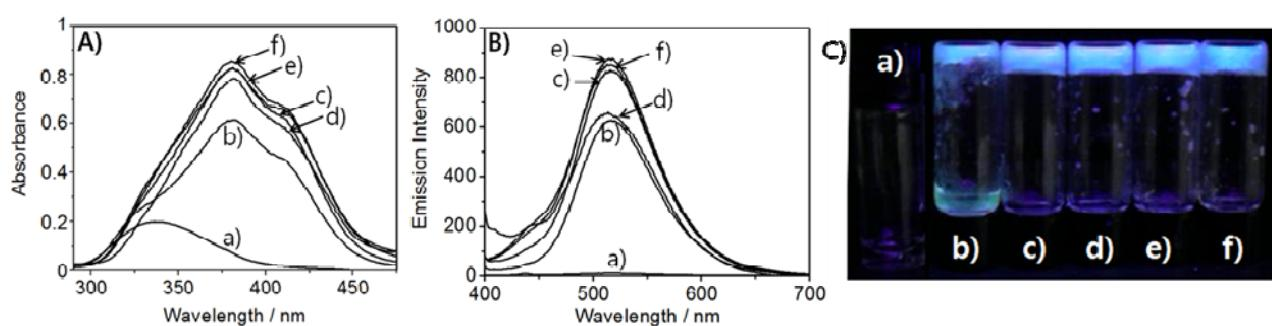
**Fig. S2** (A) UV-vis and (B) fluorescence spectra (excitation at  $\lambda=380$  nm) of (a) sol **1** (9.4 mM) and gel **1** (9.4 mM) and with (b) 1.0 equiv, (c) 2.0 equiv (d) 3.0 equiv, (e) 4.0 equiv and (f) 5.0 equiv of **2** in  $\text{H}_2\text{O}$ . (C) The photograph of (a) sol **1** (9.4 mM) and gel **1** (9.4 mM) and with (b) 1.0 equiv, (c) 2.0 equiv (d) 3.0 equiv, (e) 4.0 equiv and (f) 5.0 equiv of **2** in  $\text{H}_2\text{O}$  by irradiation of UV lamp.
