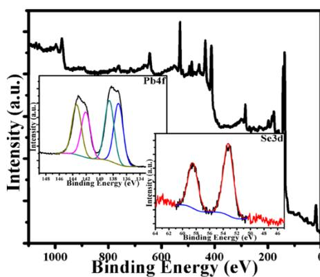
Fig. S3 XPS spectrum of PbSe NPs after illumination shows the photo corrosion of the electrode
