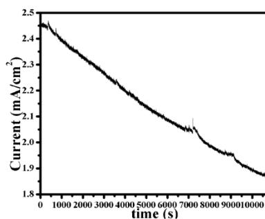
Fig. S2 Time course of photocurrent of PbSe/CdS/NT photoelectrode at -0.5 V (vs. Ag/AgCl) under simulated sun light illumination for 3 hours
