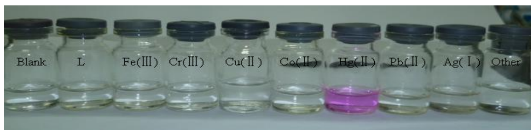
Fig.S6 Color change of the ethanol/water (4:1) solution of 3 ( 10\ \mu\text{M} ) in the presence of metal ions (20 eq)
