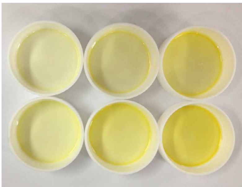
Fig. S10 Photo images of yellow free standing polymer films produced from PS/POSS-AB and PS/4- HOAB.
