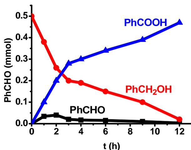
Figure 1. Distribution versus time in the oxidation of benzyl alcohol with 2.0 equiv NaOH at 60 °C.
