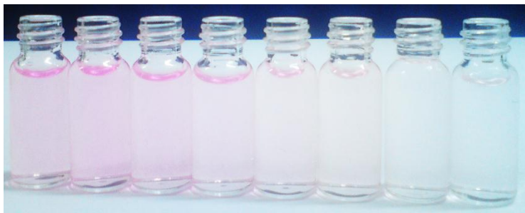
Figure S9. Colorimetric response of SS-2 (1a [25 \mu M] and p -CF 3 -PBA [50 mM]) to various concentrations of D-fructose in water/methanol (3:7, v/v, pH 5.2). [left to right: 500, 250, 100, 50, 25, 10, 5, and 1 mM]
