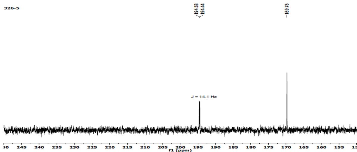
**Figure S12a.**  $^{13}\text{C}$  NMR spectrum ( $\text{CD}_2\text{Cl}_2$ ) of the reaction between MeOTf and **2d** in the carbonyl region, showing the appearance of a new signal at 194.5 ppm along with the signal of methyl acrylate at 169.8 ppm, following the addition of MeOTf.
