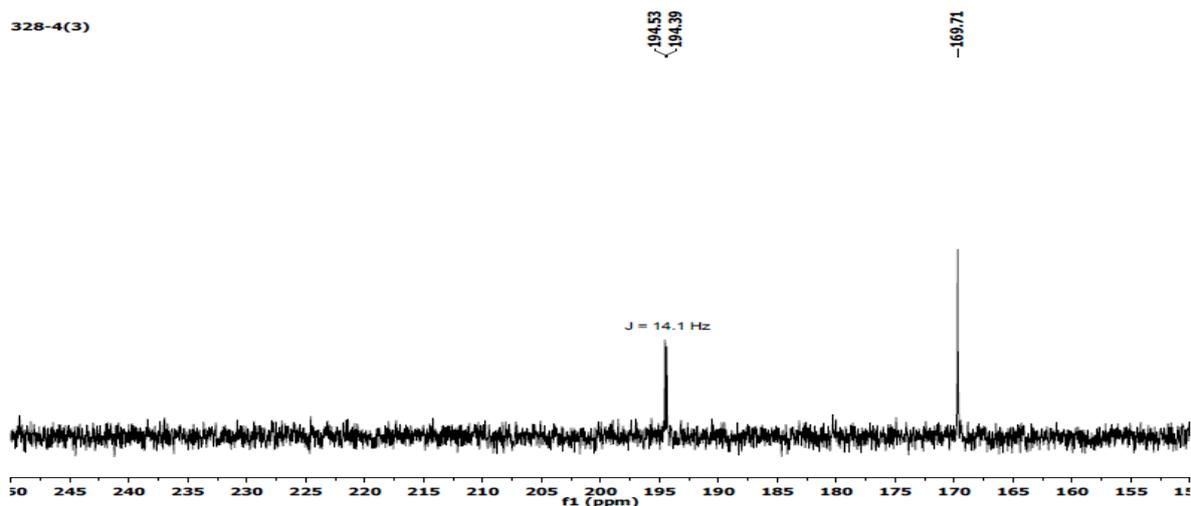
**Figure S11a.**  $^{13}\text{C}$  NMR spectrum ( $\text{CD}_2\text{Cl}_2$ ) of the reaction between MeOTf and **2c** in the carbonyl region showing the appearance of a new signal at 194.4 ppm along with the signal of methyl acrylate at 169.7 ppm, following the addition of MeOTf.
