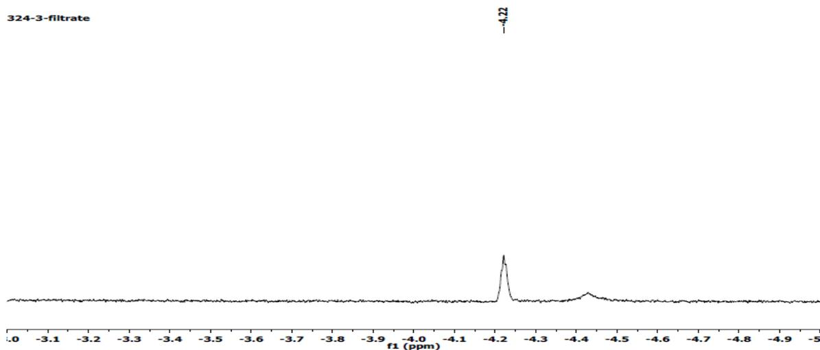
**Figure S10b.** Appearance of a new Ni-hydride species in the  $^1\text{H}$  NMR spectrum ( $\text{CD}_2\text{Cl}_2$ ) reaction of MeOTf with **2b**.
