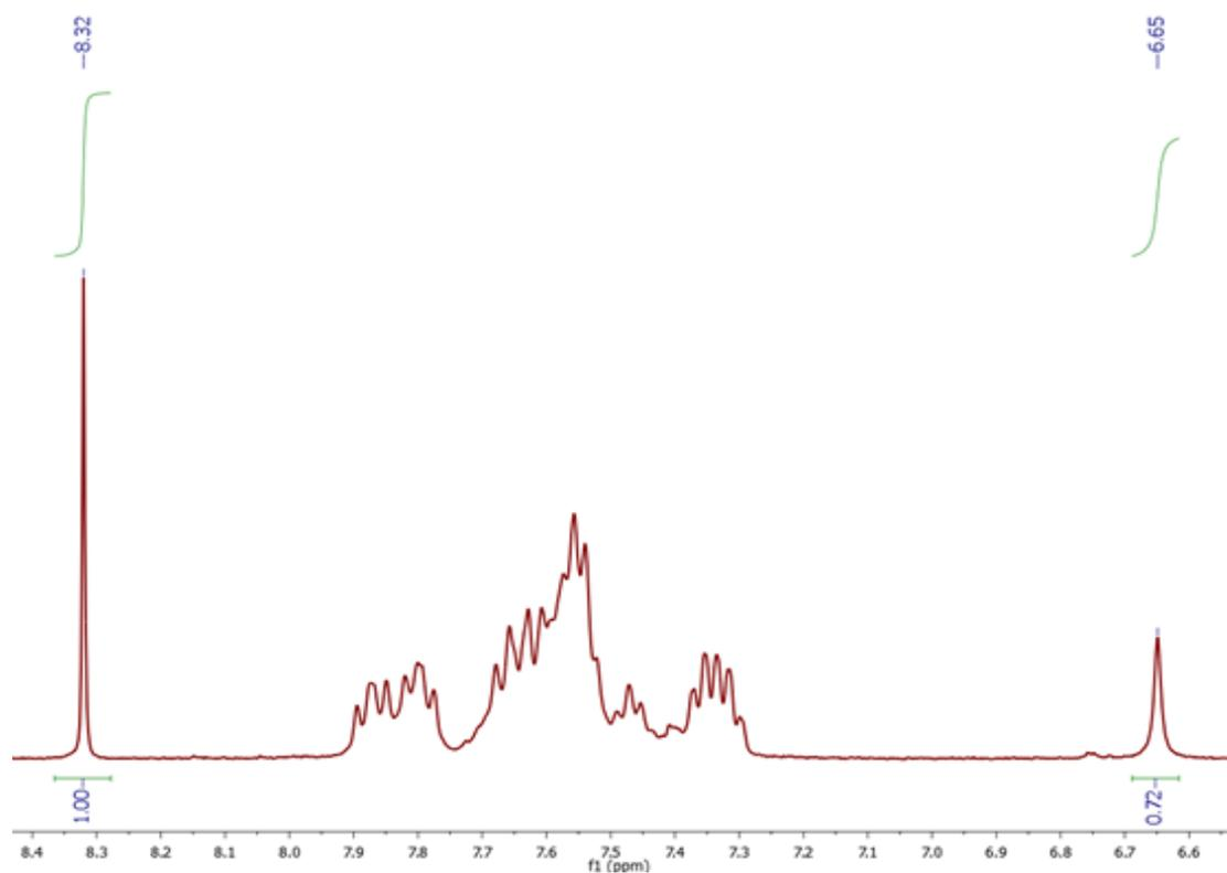
**Figure S8.**  $^1\text{H}$  NMR of the reaction between **7b** and MeOTf (2 equiv. MeOTf, 15 min, using  $\text{CH}_3\text{Cl}$  as a standard in  $\text{DMSO}-d_6$ , the concentration of the standard is equimolar to the initial concentration of **7b**) to afford **8c**.
