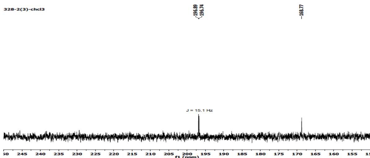
**Figure S9a.**  $^{13}\text{C}$  NMR spectrum ( $\text{CD}_2\text{Cl}_2$ ) of the reaction between MeOTf and **2a** in the carbonyl region showing the appearance of a new signal at 196.7 ppm along with the signal of methyl acrylate at 168.8 ppm, following the addition of MeOTf.
