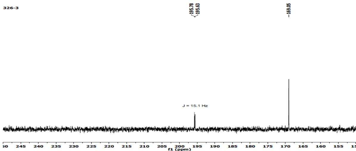
**Figure S10a.**  $^{13}\text{C}$  NMR spectrum ( $\text{CD}_2\text{Cl}_2$ ) of the reaction between MeOTf and **2b** in the carbonyl region showing the appearance of a new signal at 195.7 ppm along with the signal of methyl acrylate at 169.0 ppm, following the addition of MeOTf.
