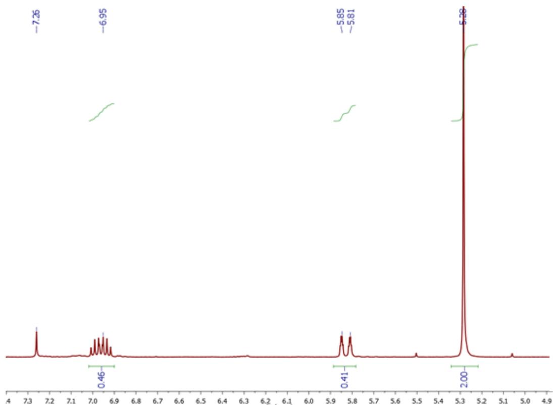
**Figure S7.**  $^1\text{H}$  NMR of the reaction between **7a** and MeOTf (100 equiv. MeI, 3 h, in  $\text{CDCl}_3$  with  $\text{CH}_2\text{Cl}_2$  as internal standard, the concentration of the standard is 1/2 of the initial concentration of **7a**) to afford **8a** selectively.
