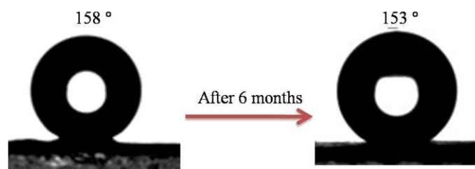
Fig. S4 The water droplet shapes of the as-prepared superhydrophobic PMMA surface before and after it was placed under the air condition for 6 months. The surface can still keep superhydrophobicity with a WCA of 153° after 6 months.
