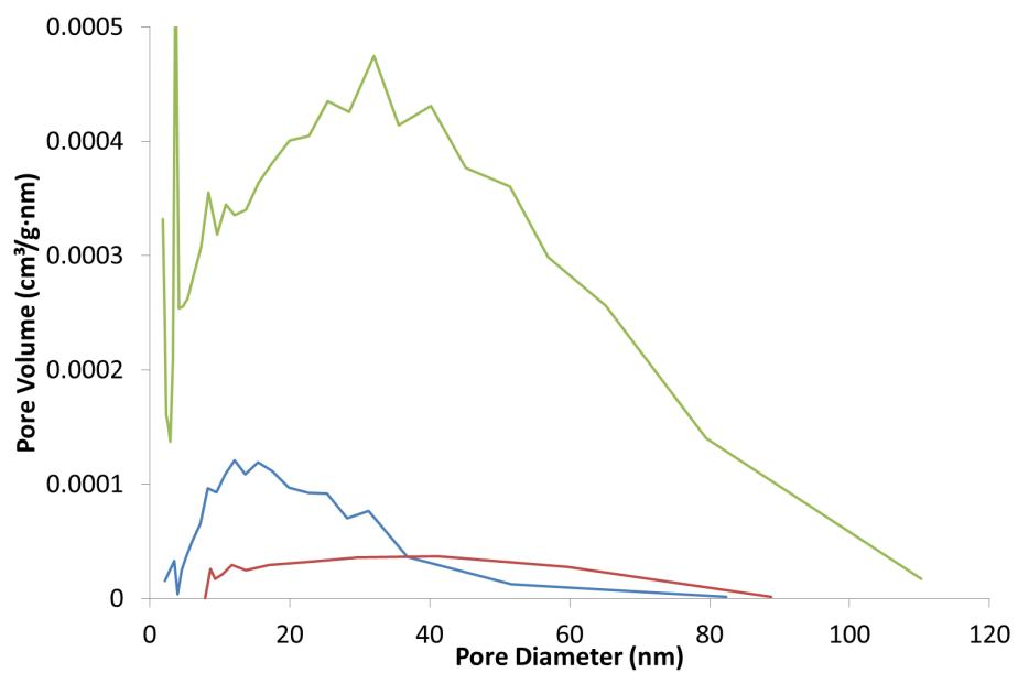
**Figure S11** Pore size distribution calculated from the desorption isotherm measured for washed polymer samples templated with **1**: 1 % w/v (blue), 5 % w/v (red), 10 % w/v (green).
