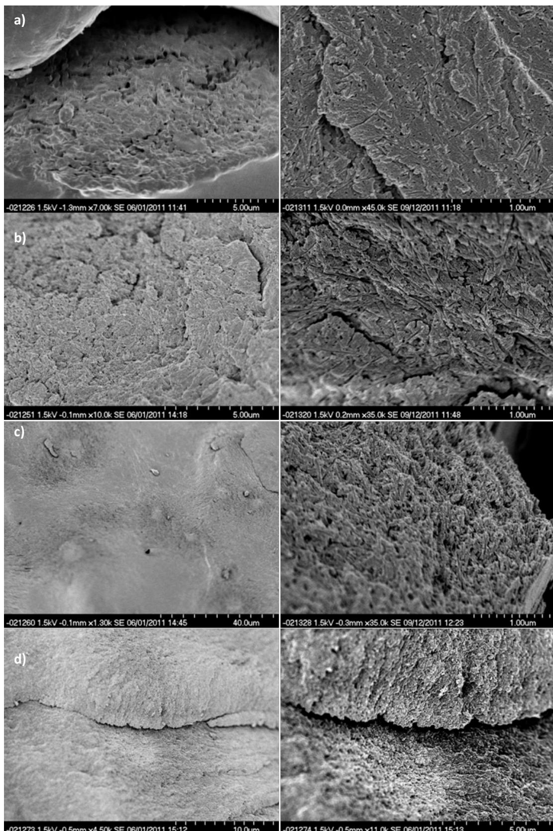
**Figure S6** SEM images of washed polymers formed from a) 1 wt%, b) 5 wt%, c) 10 wt% and d) 20 wt% of gelator **2** in polymerised 1:1 MMA:EGDMA following washing with methanol.
