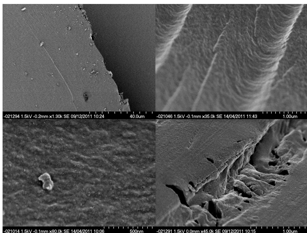
**Figure S8** SEM images of control polymer formed from 1:1 MMA:EGDMA without gelator
