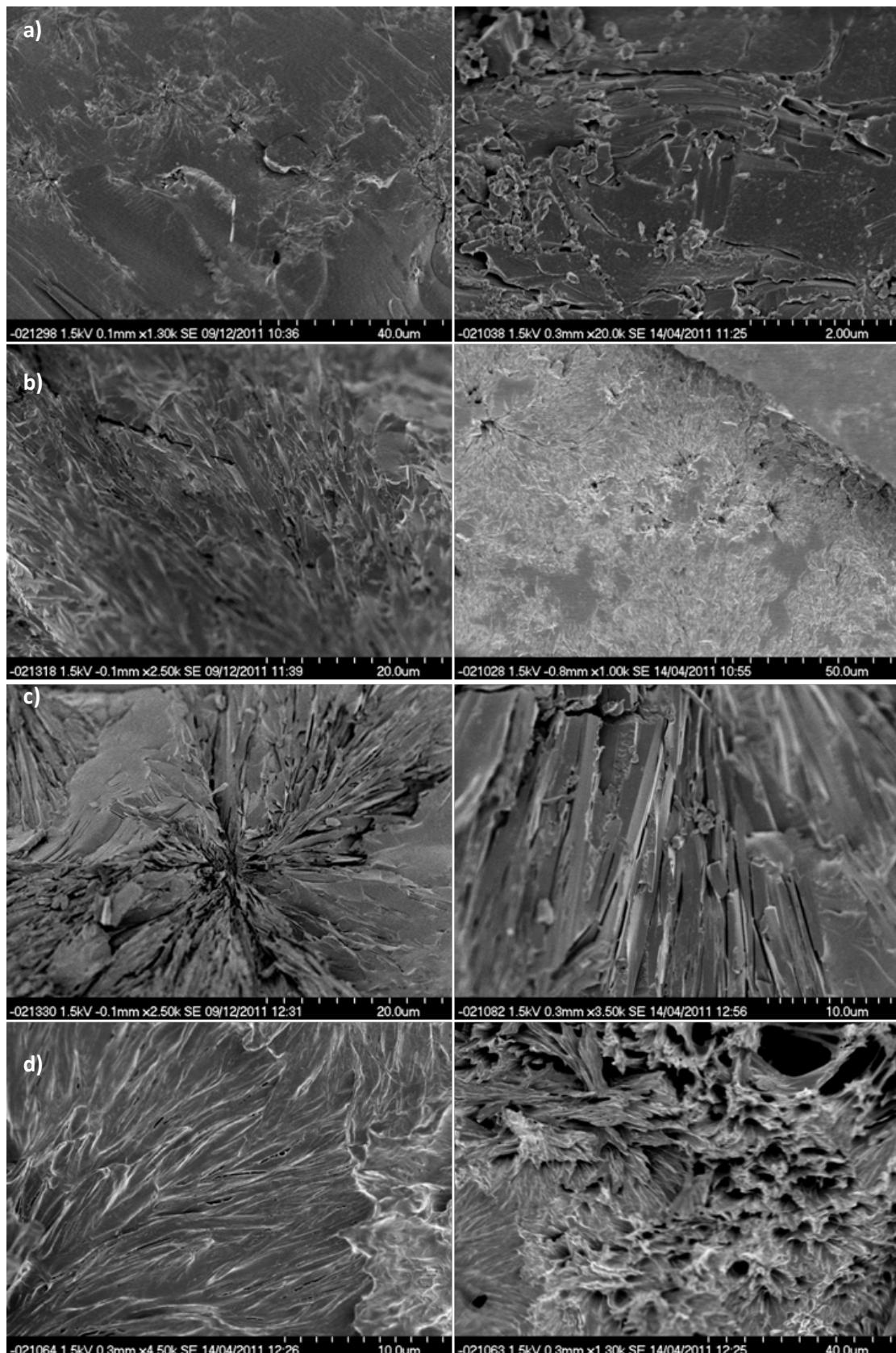
**Figure S5** SEM images of washed polymers formed from a) 1 wt%, b) 5 wt%, c) 10 wt% and d) 20 wt% of gelator **1** in polymerised 1:1 MMA:EGDMA.
