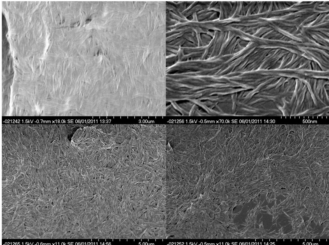
**Figure S2** SEM images of xerogels formed from a) 2 wt%, b) 5 wt%, c) 10 wt% and d) 20 wt% of gelator **1** in 1:1 MMA:EGDMA
