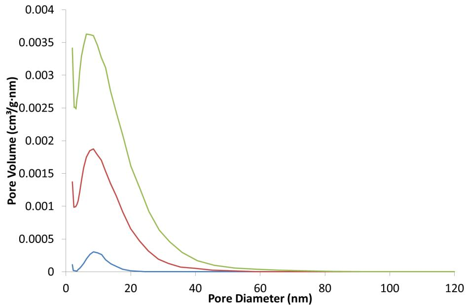
**Figure S10** Pore size distribution calculated from the adsorption isotherm measured for washed polymer samples templated with **2**: 1 % w/v (blue), 5 % w/v (red), 10 % w/v (green).
