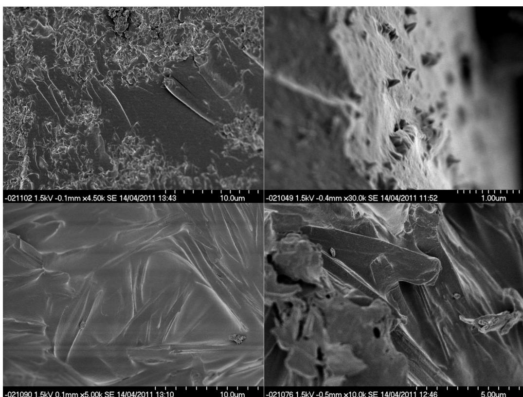
**Figure S3** SEM images of composite gels formed from a) 2 wt%, b) 5 wt%, c) 10 wt% and d) 20 wt% of gelator **1** in polymerised 1:1 MMA:EGDMA.
