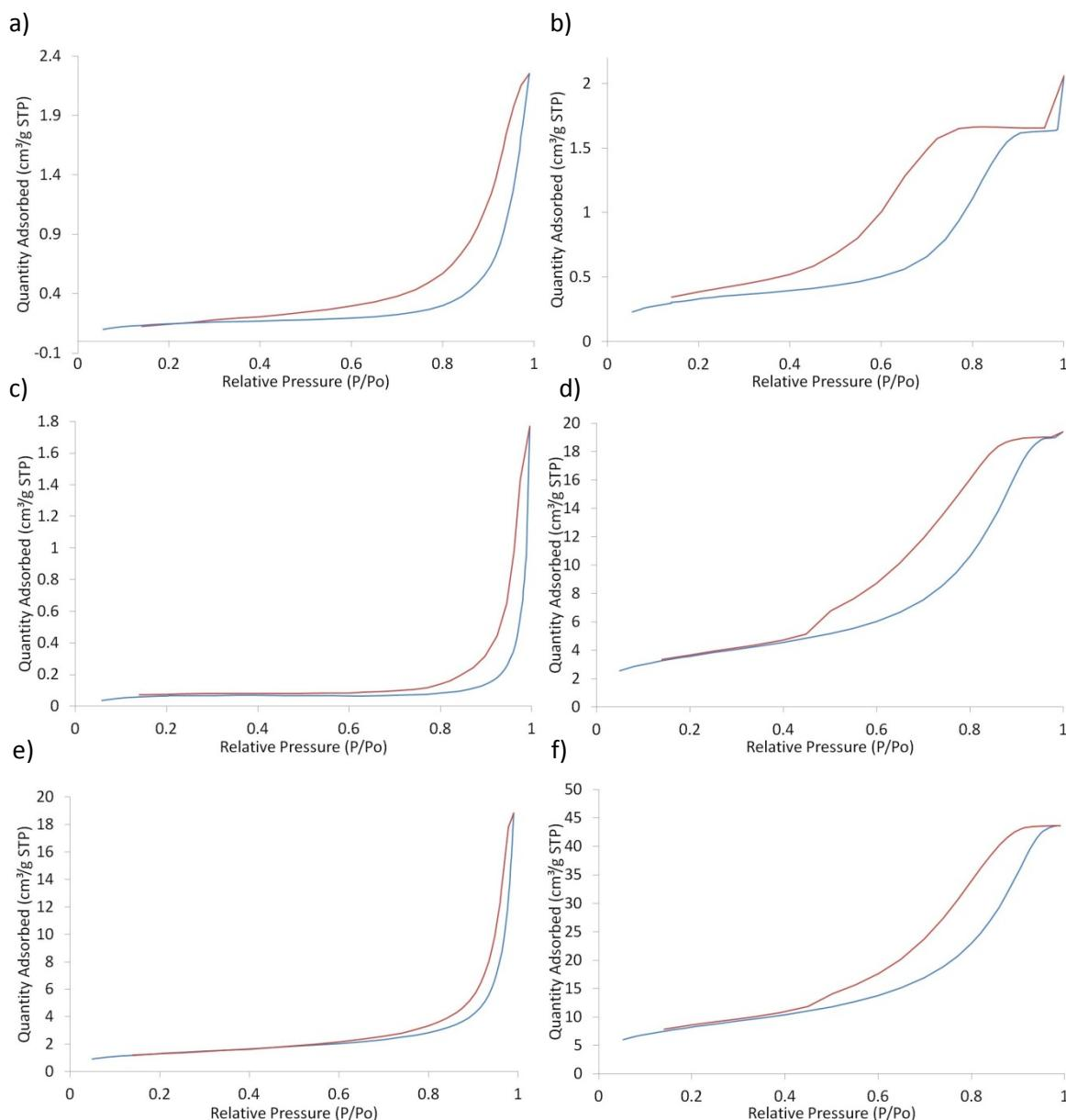
**Figure S9** BET isotherms showing adsorption (blue) desorption (red) curves for washed polymer samples formed from a) 1 % w/v **1** b) 1 % w/v **2** c) 5 % w/v **1** d) 5 % w/v **2** e) 10 % w/v **1** f) 10 % w/v **2**
