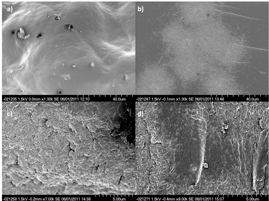
**Figure S4** SEM images of composite gels formed from a) 2 wt%, b) 5 wt%, c) 10 wt% and d) 20 wt%. of gelator **2** in polymerised 1:1 MMA:EGDMA.
