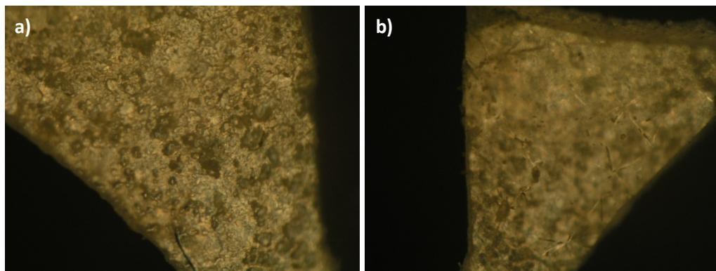
**Figure S7** Optical microscopy images showing different faces of polymer sample a) rough face, b) smooth face
