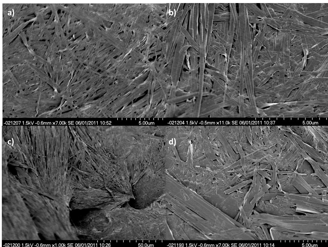
**Figure S1** SEM images of xerogels formed from a) 2 wt%, b) 5 wt%, c) 10 wt% and d) 20 wt% of gelator **1** in 1:1 MMA:EGDMA
