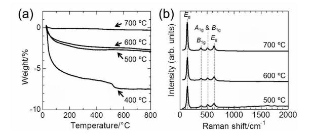
Figure S1 (a) TG curves and (b) Raman spectra of the samples calcined at different temperatures.
