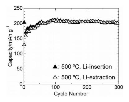
Figure S2 Cycle performance of the sample calcined at 500 °C at 100 mA g<sup>-1</sup>.
