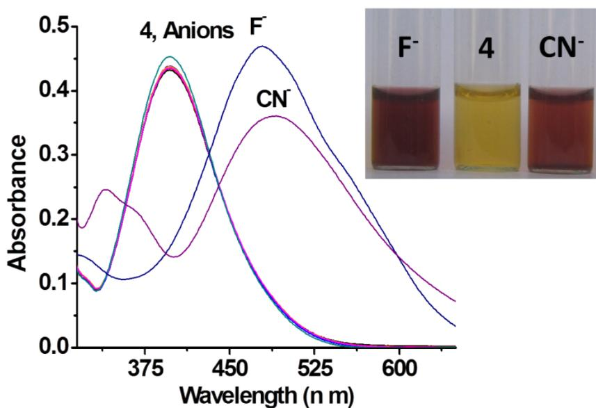
**Figure S14:** Change in absorption spectra of **4** (10  $\mu\text{M}$ ) upon addition of various anions (5 equiv) in MeCN. Inset shows the change in color of solution upon addition of  $\text{F}^-$  and  $\text{CN}^-$  ions.
