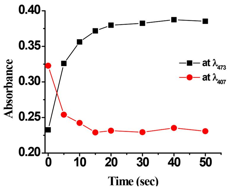
**Figure S16:** Response time curve evaluated through UV-Vis absorption response of **4** (10  $\mu$ M) upon addition of 2 equiv of  $\text{CN}^-$  in aqueous-MeCN (50%, v/v).
