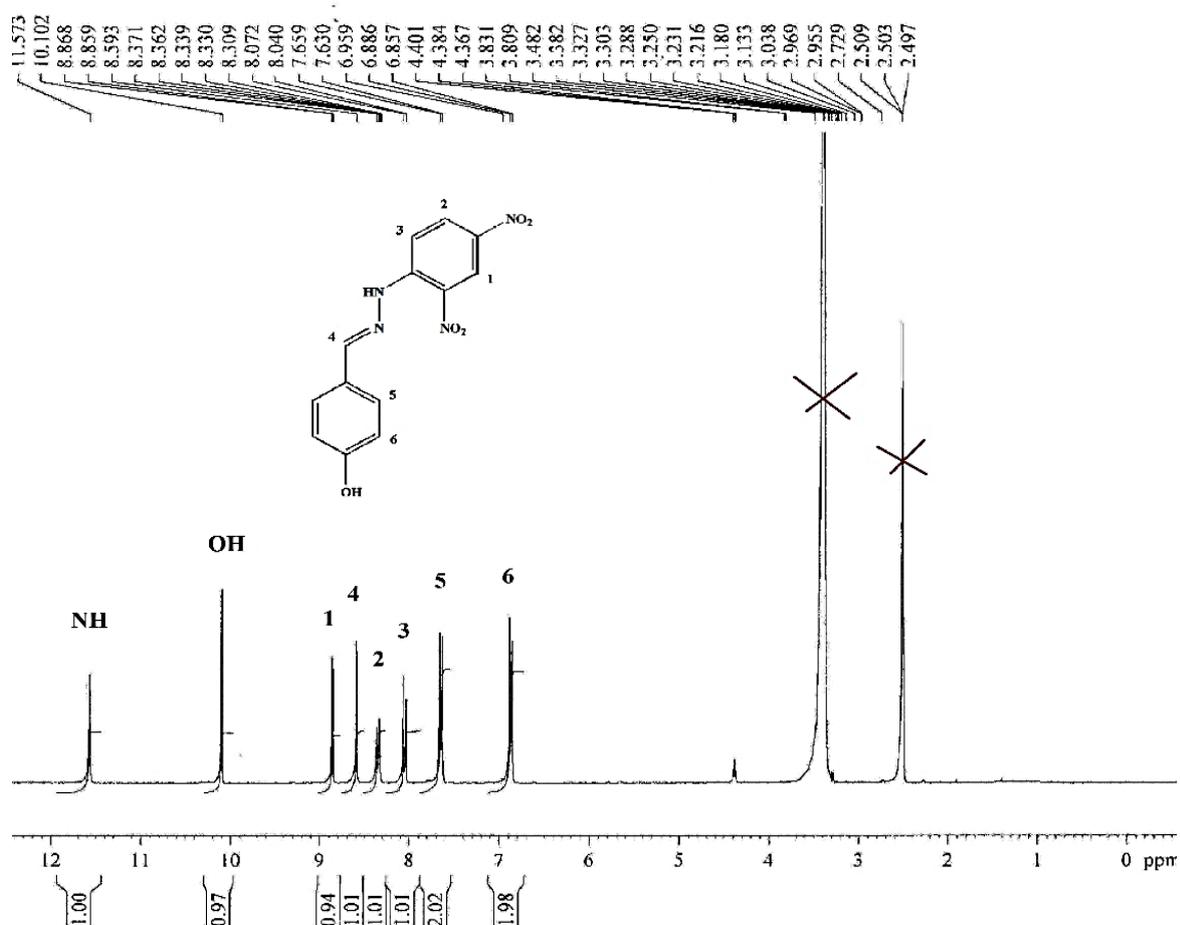
**Figure S13:** <sup>1</sup>H NMR spectrum of **Model** compound in DMSO-*d*<sub>6</sub>.
