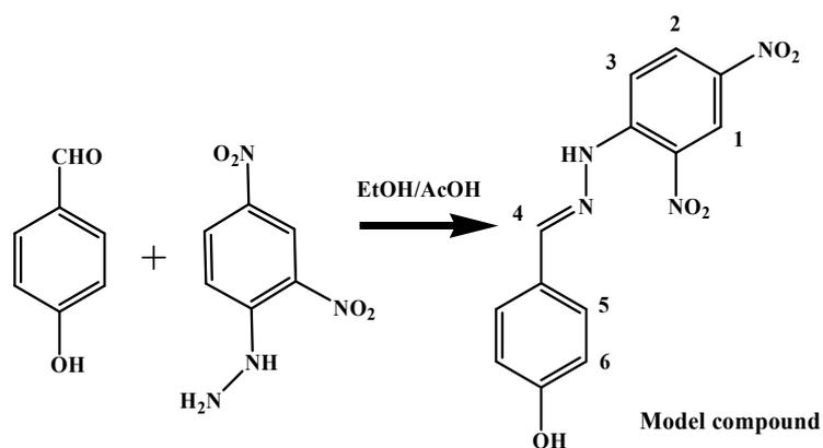
**Scheme S1:** Synthesis of phenolic hydrazone model compound.
