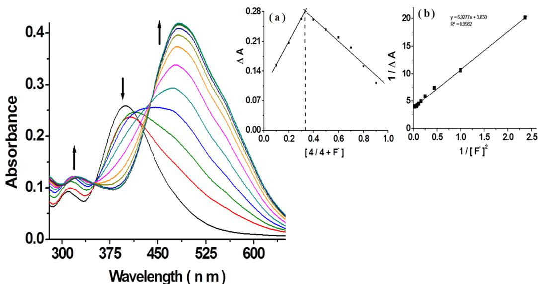
**Figure S15:** Absorption titration spectrum of **4** (10  $\mu\text{M}$ ) upon addition of  $\text{F}^-$  ions (0 – 5 equiv) in MeCN. Inset: (a) Jobs Plot and (b) B-H plot of **4** for  $\text{F}^-$ .
