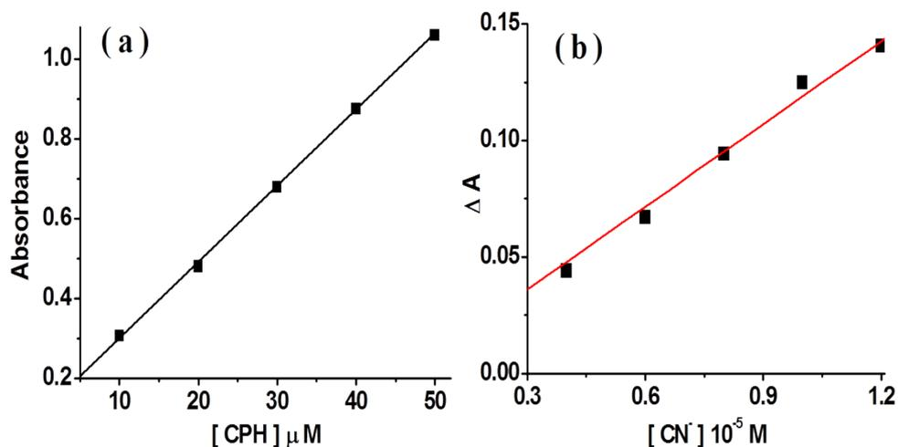
**FigureS11:** (a) Calibration curve for **4** and (b) calibration sensitivity of CN<sup>-</sup> ion in aqueous-MeCN (50%, v/v).
