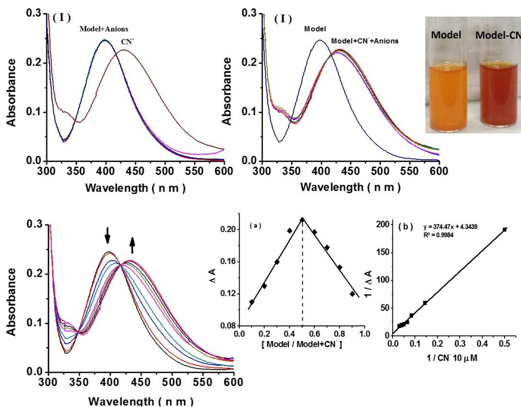
**Figure S12:**(I) Change in the absorption spectra of phenolic hydrazone model compound ( $10 \mu\text{M}$ ) on addition of various anions (50 equiv) in aqueous-MeCN (50%, v/v) and (II) Studies on interference of different ions when interacted with the model compound and change in color of the solution. Absorption titration spectrum of model compound. Inset shows (a) Job's plot, (b) B-H plot.
