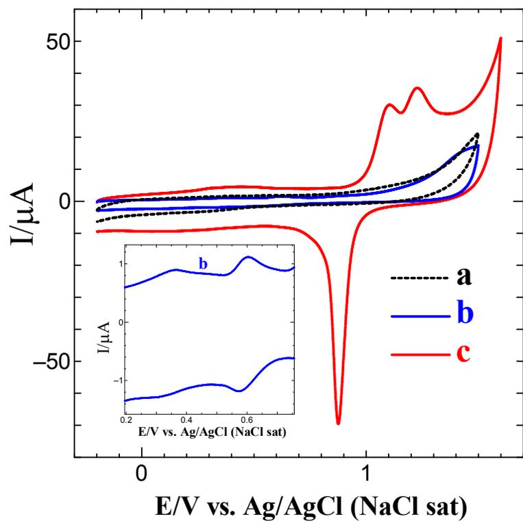
**Fig. S3** CVs obtained for (a) bare GCE, (b) GCE/Co(II)MTpAP and (c) GCE/Co(II)MTpAP/cit-AuNPs in 0.1 M  $\text{H}_2\text{SO}_4$  at a scan rate of  $0.1 \text{ V s}^{-1}$ .
