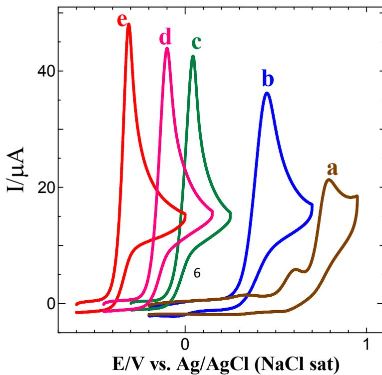
**Fig. S6** CVs obtained for 0.5 mM hydrazine in pH (a) 2, (b) 4, (c) 7, (d) 9 and (e) 12 at GCE/Co(II)MTpAP/cit-AuNPs at a scan rate of  $0.05 \text{ V s}^{-1}$ .
