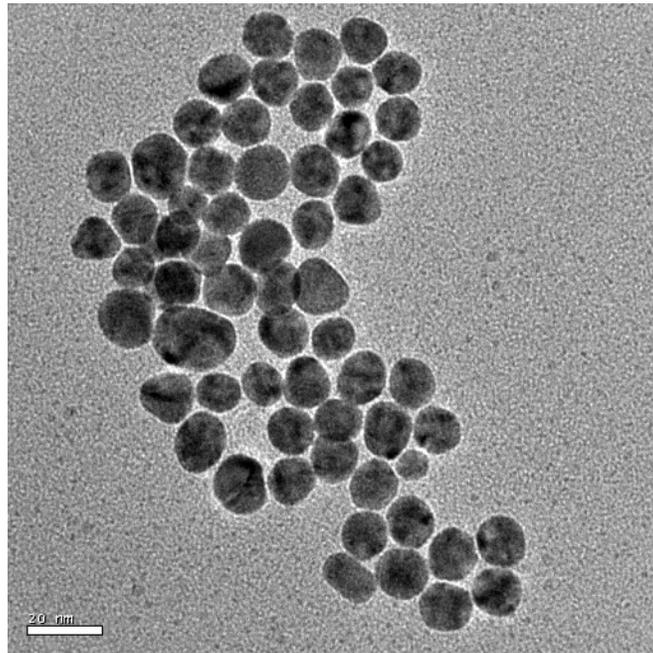
**Fig. S2** TEM image obtained for colloidal cit-AuNPs.
