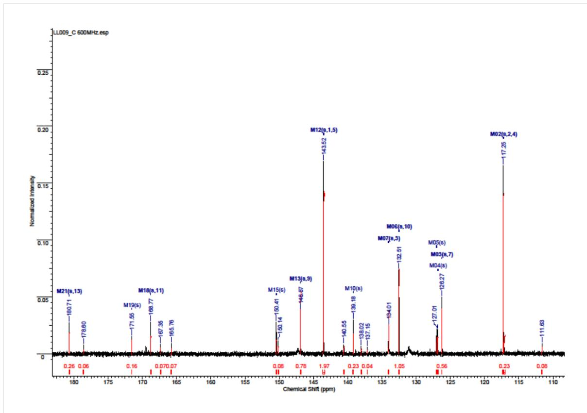
**Figure S21** Zoomed in view of  $^{13}\text{C}$  NMR spectrum for **4** showing chemical shifts in the area 110-180 ppm
