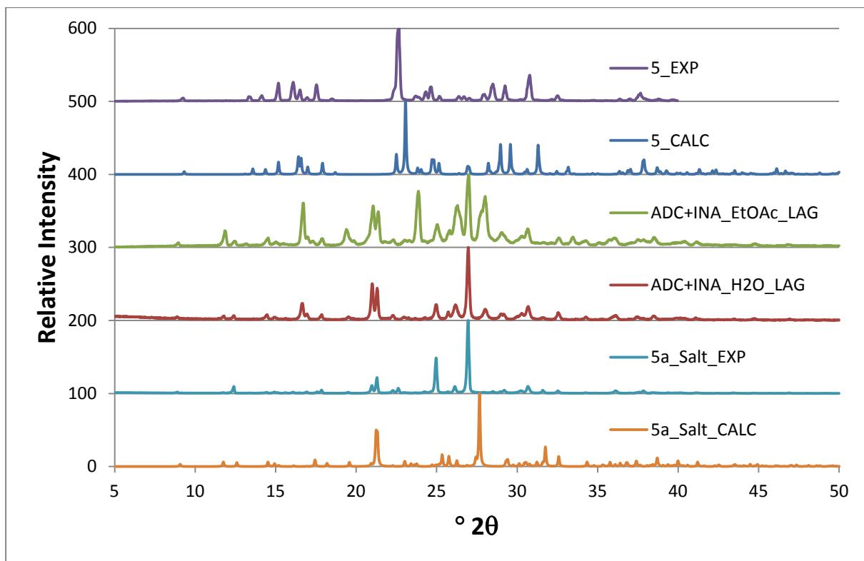
**Figure S15** Experimental and calculated PXRD patterns for **5** and **5a** compared to the products obtained from liquid-assisted grinding (LAG) experiments using either ethyl acetate (EtOAc) or water (H<sub>2</sub>O) as solvent.
