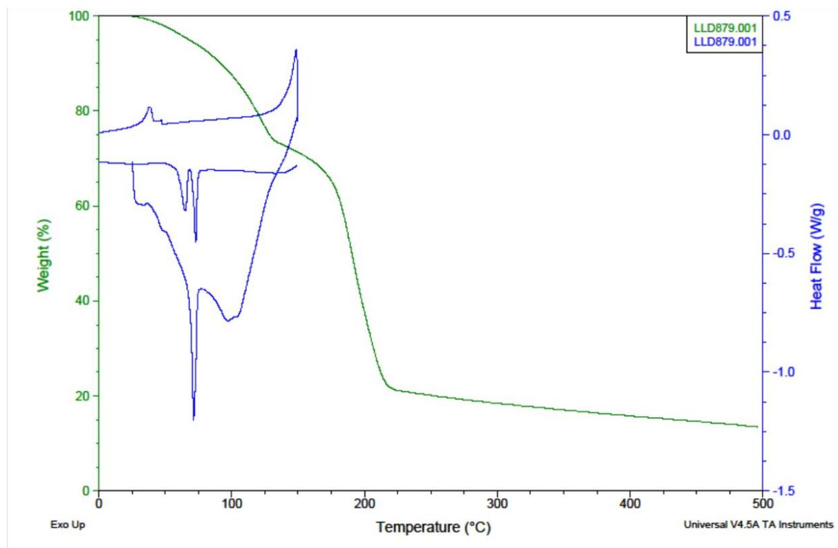
**Figure S9** DSC (blue) and TG (green) analysis of **6a**. TGA shows a large mass loss (27%) starting at ambient temperature.
