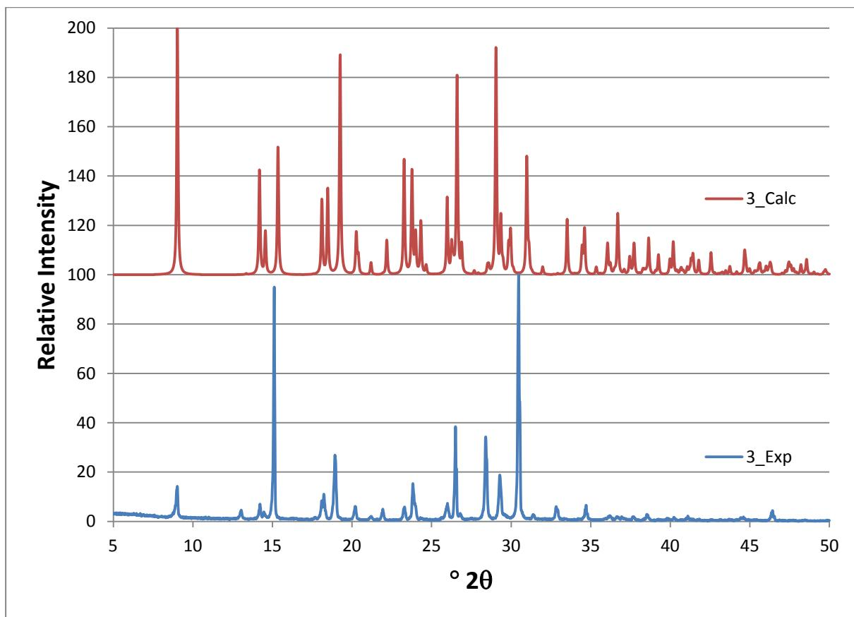
**Figure S13** Calculated (red) and experimental (blue) PXRD patterns for compound 3
