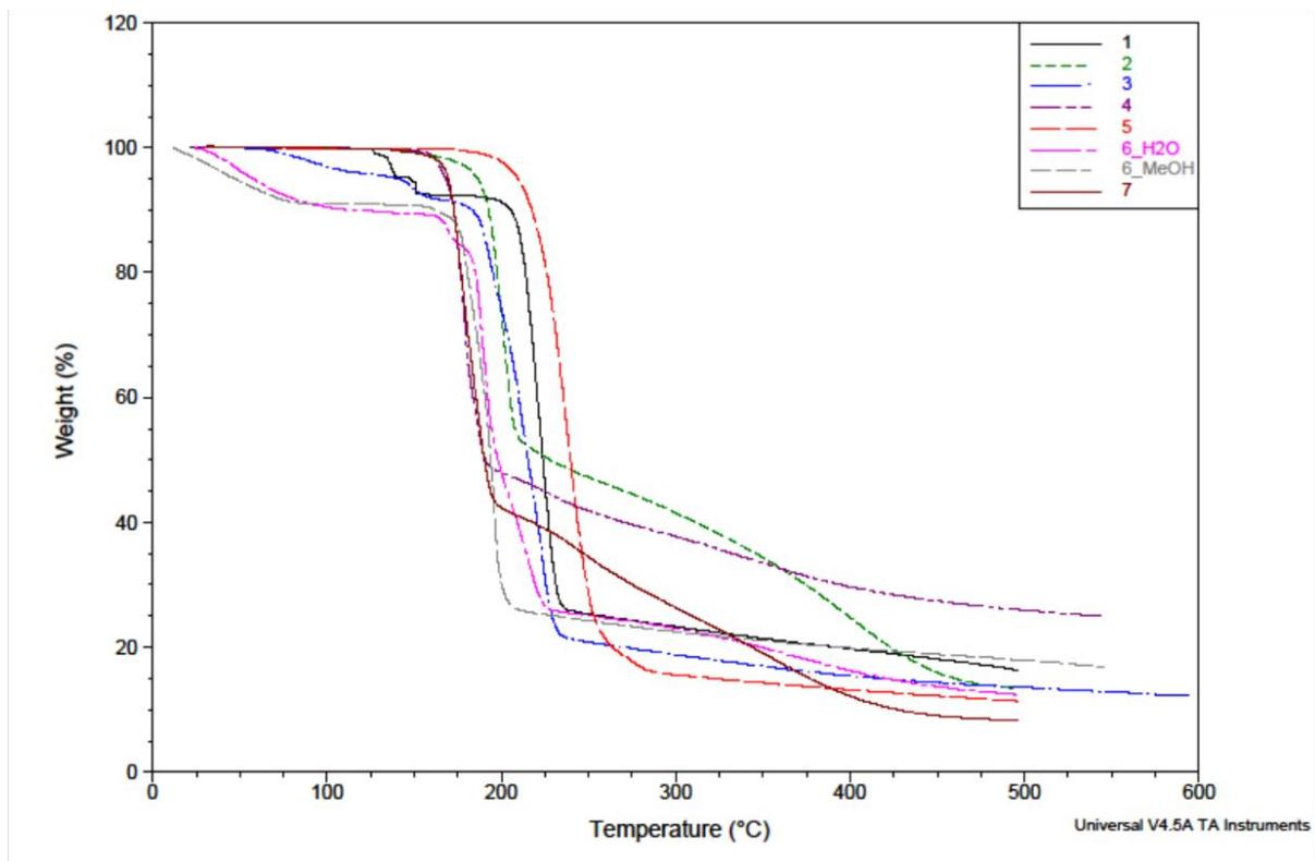
Figure S1 Overlay of TGA analysis of compounds 1-7.
