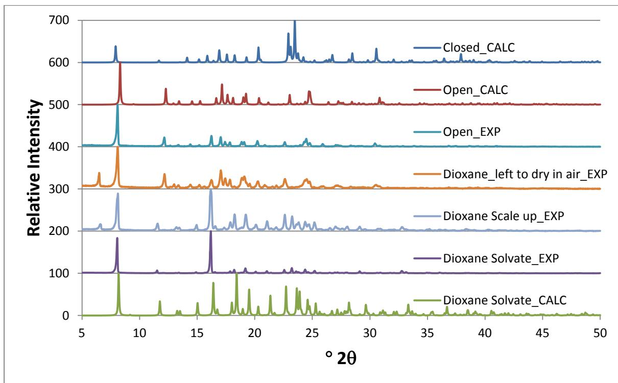
**Figure S17** Comparison of experimental and calculated PXRD patterns for **7** (calc), **7<sub>open</sub>**, **7<sub>diox</sub>** and **7<sub>diox</sub>** that was left in air for approximately 3 weeks
