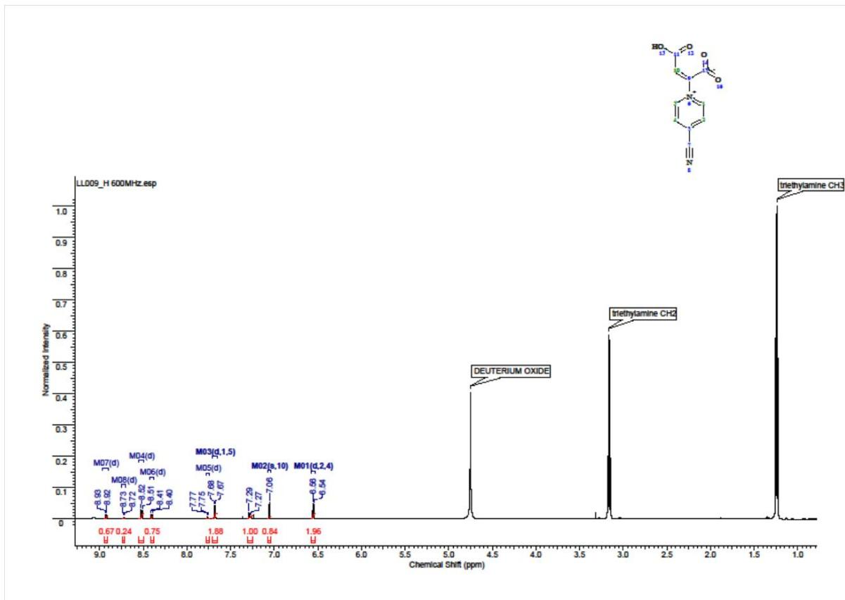
**Figure S18**  $^1\text{H}$  NMR spectrum for **4**, the zwitteric compound was identified by comparing the ratio of the intergrals of the resonance peaks.
