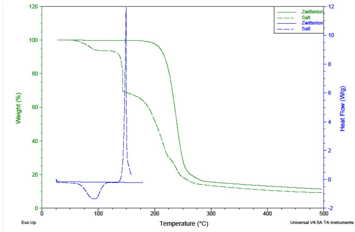
Figure S6 DSC (blue) and TG (green) analysis of **5** (solid line) and **5a** (dotted line).
