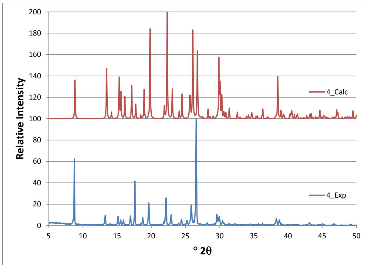
**Figure S14** Calculated (red) and experimental (blue) PXRD patterns for compound 4
