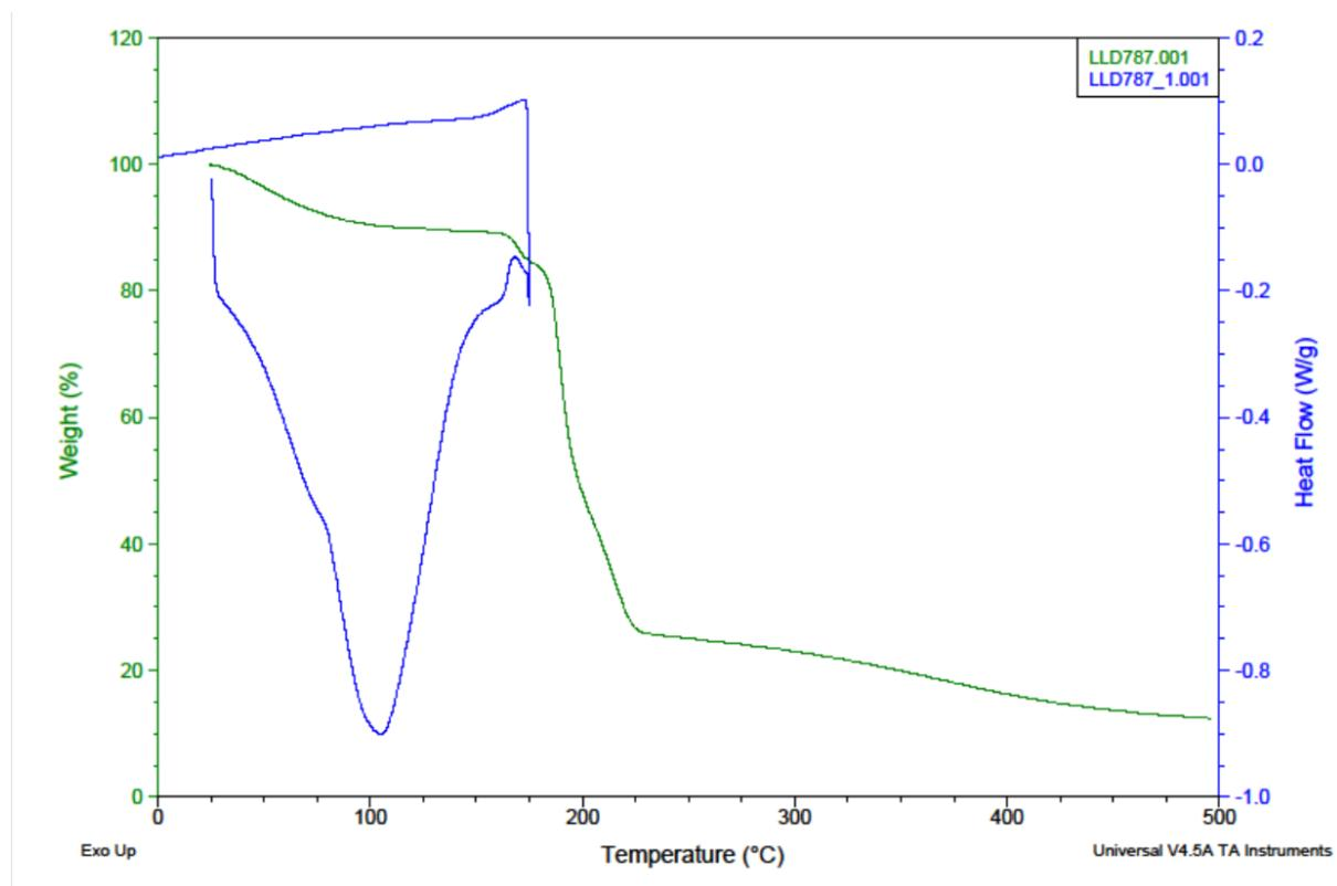
**Figure S7** DSC (blue) and TG (green) analysis of **6**·H<sub>2</sub>O, 11.02% weight loss corresponds to the expected 11.1% for two molecules of water per 1 molecule of **6** as observed in the crystal structure (two partially occupied molecules).
