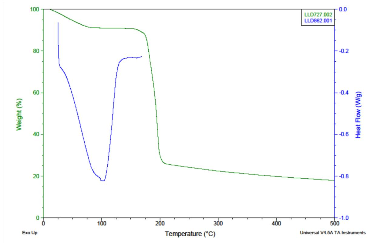
**Figure S8** DSC (blue) and TG (green) analysis of **6**·MeOH. The TGA shows a 9.2% mass loss which corresponds to one methanol molecule per host molecule. This corresponds well with the crystal structure data.
