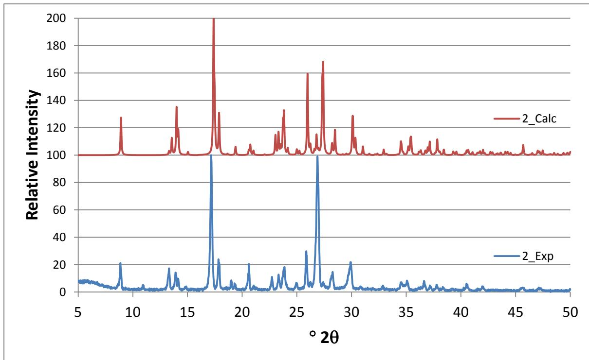
Figure S12 Calculated (red) and experimental (blue) PXRD patterns for compound **2**.
