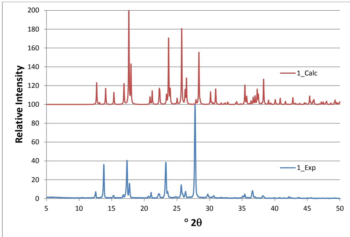
Figure S11 PXRD patterns for **1**, calculated (red) and experimental (blue)
