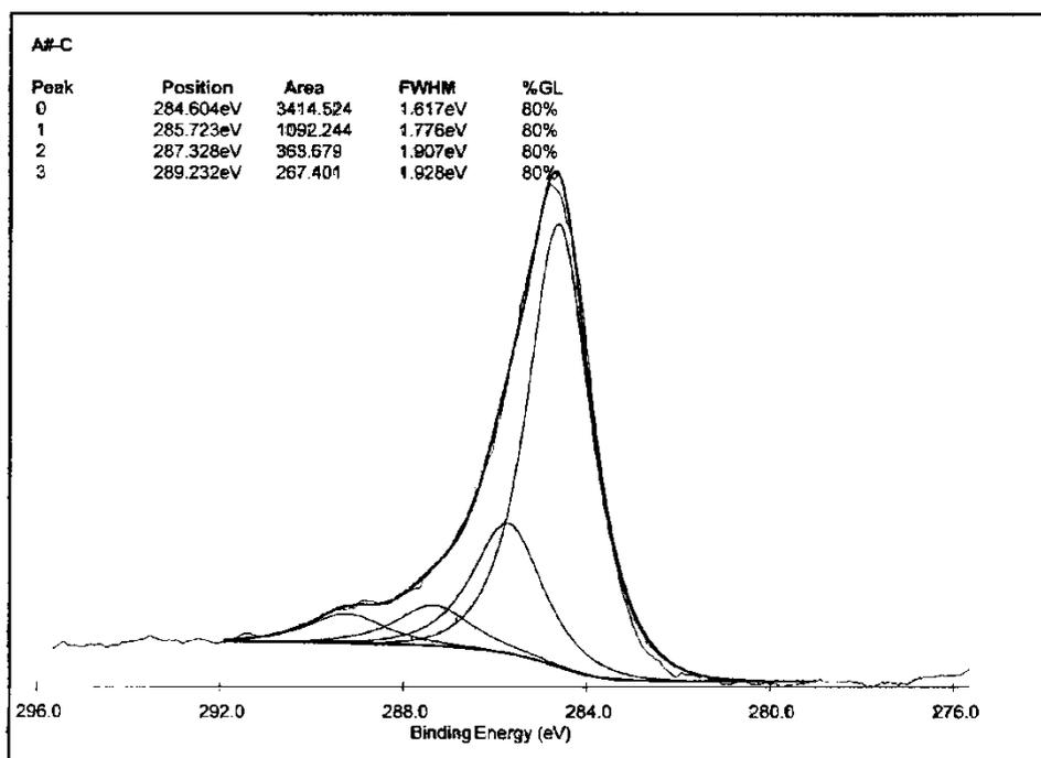
**Figure 1** High-resolution C1s XPS survey for the nitrogen-graphene pyrolysed from CuPc molecular under Ar atmosphere on the ceramic griddle.
