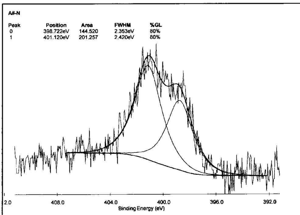
**Figure 2** High-resolution N1s XPS survey for the nitrogen-graphene pyrolysed from CuPc molecular under Ar atmosphere on the ceramic griddle.
