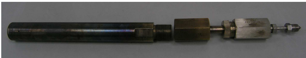
Fig. S1 Model HR-1B-2, LECO hydrothermal synthesis reactor
