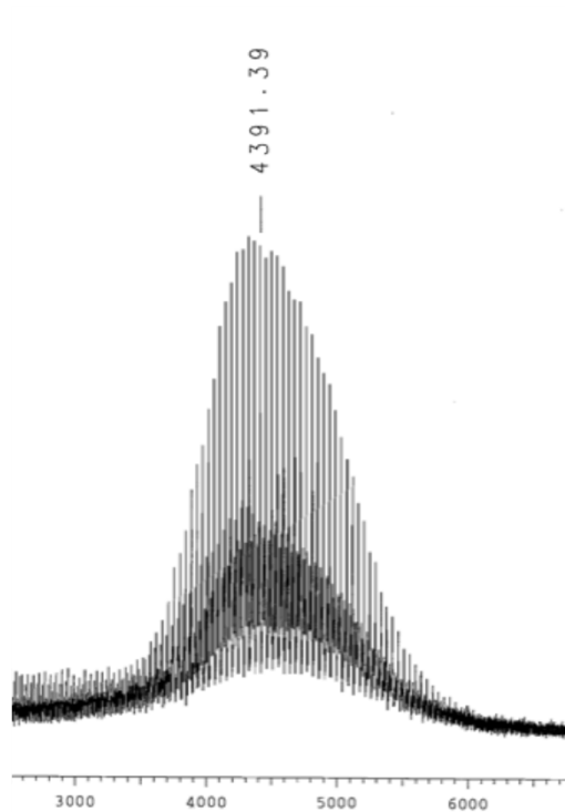
Figure S16: Mass spectrum of DOUPEG3000-FA 4 with a peak at the m/z range around 4391.
