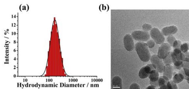
**Fig. S8.** The nanodevices were stable in 10mM PBS. They were well distributed in PBS for one month without significant changes to their size (a) and morphology (b).
