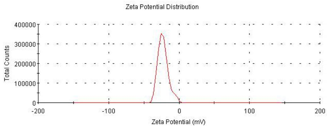
**Fig. S6.** Zeta potential distribution of MSN@p(NIPAM-*co*-MA) in distilled H<sub>2</sub>O.
