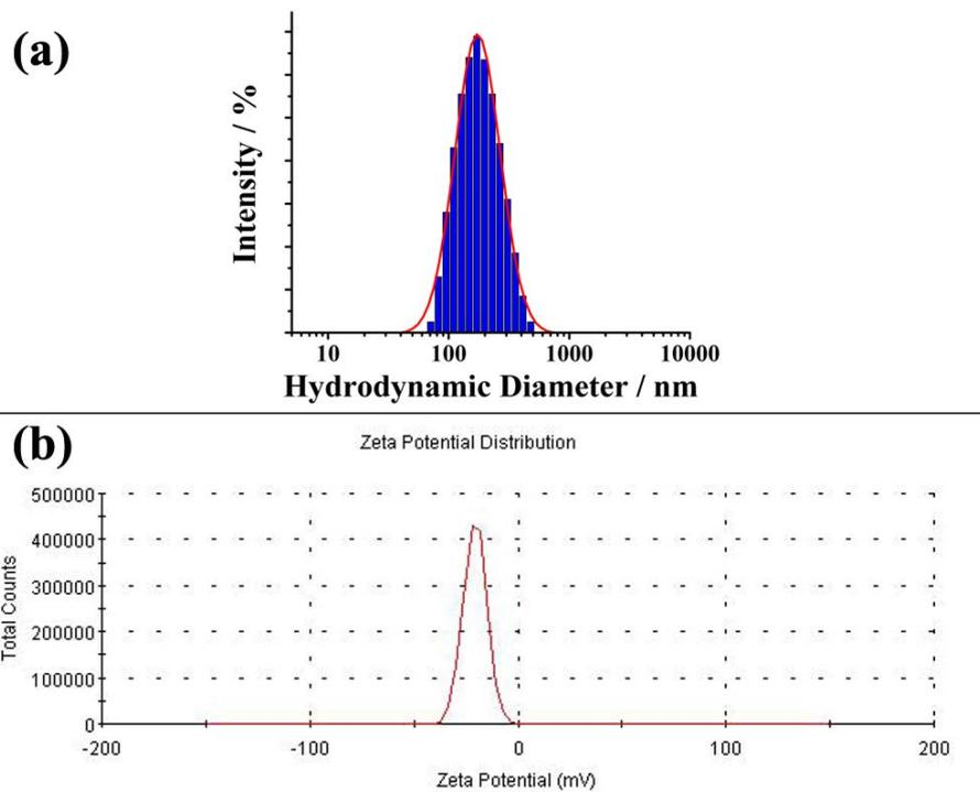
**Fig. S9.** (a) Hydrodynamic diameter and (b) Zeta potential distribution of the nanocarriers after drug loading. No significant changes were observed.
