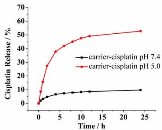
**Fig. S10.** Release profiles of cisplatin-loaded MSN@p(NIPAM-co-MA)-FA in response to pH at room temperature.
