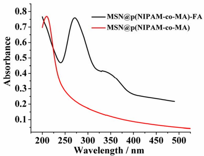
**Fig. S7.** UV-vis absorption spectra of MSN@p(NIPAM-co-MA) and MSN@p(NIPAM-co-MA)-FA.
