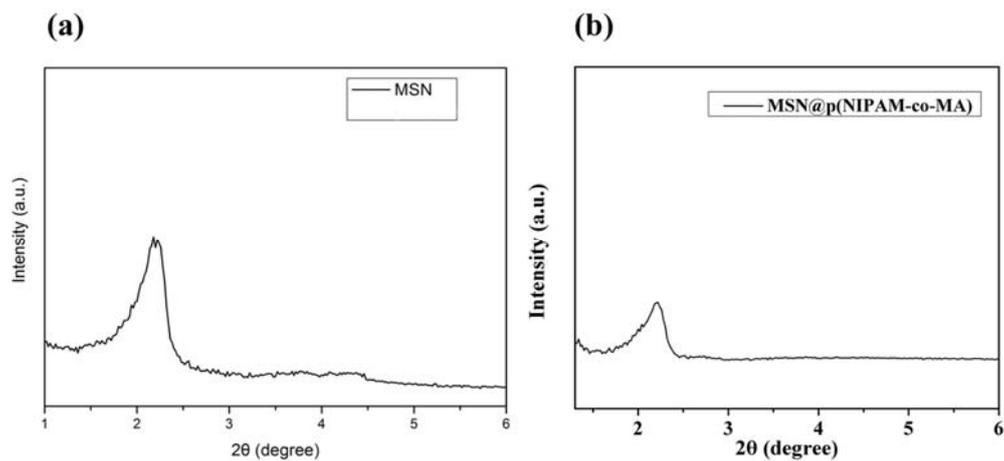
**Fig. S4.** Low-angle XRD pattern revealed that (a) MSNs exhibited a well-ordered porous structure with a hexagonal arrangement, (b) MSN@p(NIPAM-co-MA) still remained mesoporous despite the lower intensity of XRD peaks, which may be ascribed to the capping effect.
