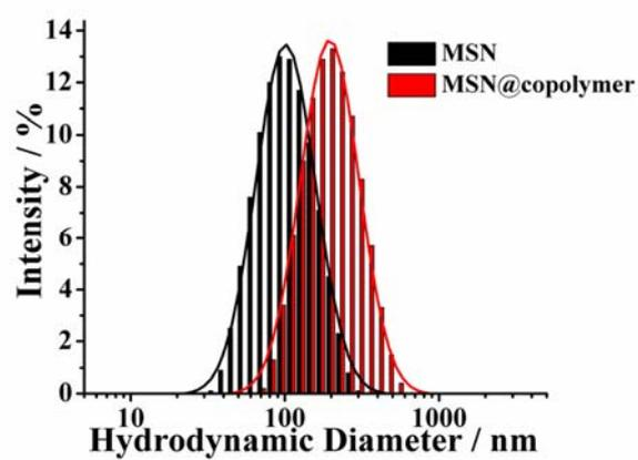
**Fig. S5.** Hydrodynamic diameter of MSN and MSN@p(NIPAM-*co*-MA).
