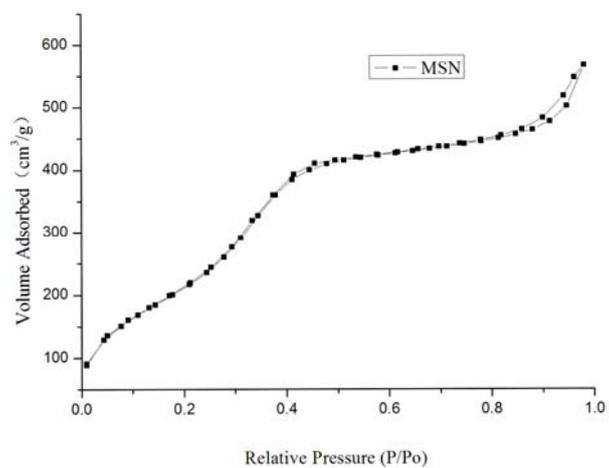
**Fig. S3.** Nitrogen adsorption desorption isotherms and Brunauer–Emmett–Teller (BET) analysis indicated specific surface area of 786 m<sup>2</sup>g<sup>-1</sup>.
