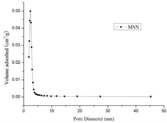
**Fig. S2.** Pore size distribution curve derived from desorption isotherm measurements and Barret–Joyner–Halenda (BJH) analysis indicated an average pore diameter of 2.5 nm.
