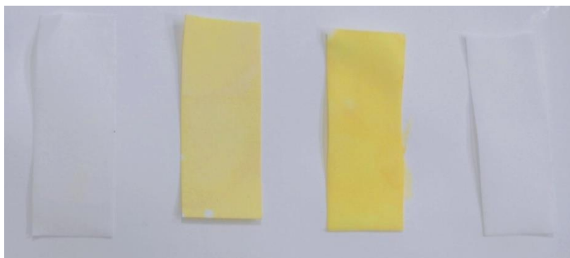
Figure S15: Dye coated filter paper in acidic, neutral, basic and acidic (reversibility from basic medium) (from left to right)
