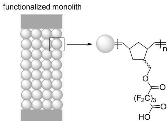
Preparation of the monolithic support inside a PEEK column (100 x 7 mm i.d.) and grafting of functionalized monomer **M1** (~ 120  $\mu\text{mol}$ ) to the monolithic support was performed according to literature procedures.<sup>4</sup>
