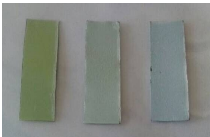
Figure S4. Photographs of blank TiO 2 NBs ( right: white ), TiO 2 NBs/CdS QDs ( middle: light yellow ), and TiO 2 NBs-CdS QDs heterostructure ( left: yellow ).
