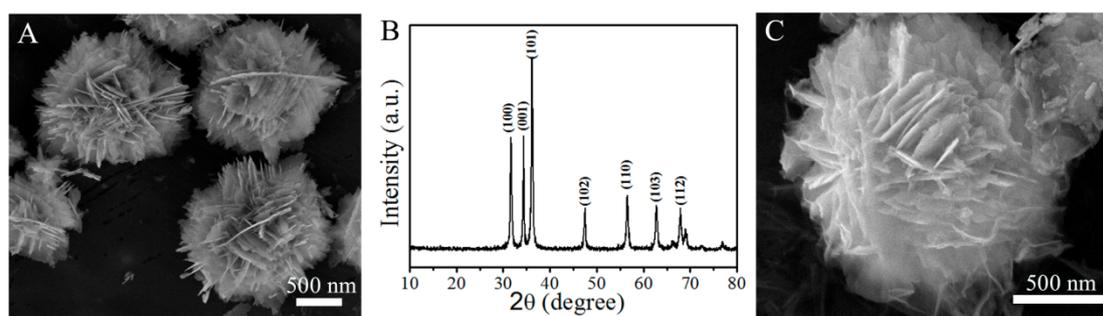
**Fig. S1.** (A) SEM image and (B) XRD of the F-ZnO; (C) SEM image of the F-ZnO covered with carbon material.
