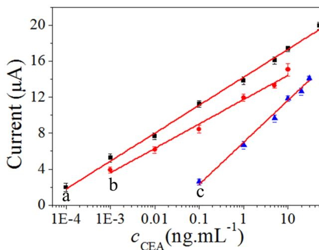
**Fig. S3.** Calibration curves of the electrochemical immunosensor toward CEA standards in pH 7.4 PBS containing 50  $\mu\text{mol}\cdot\text{L}^{-1}$  TH and 3  $\text{mmol}\cdot\text{L}^{-1}$  H<sub>2</sub>O<sub>2</sub> with different labels: (a) AuNPs/FCM, (B) AuNPs/carbon sphere, (c) AuNPs/graphene sheets.
