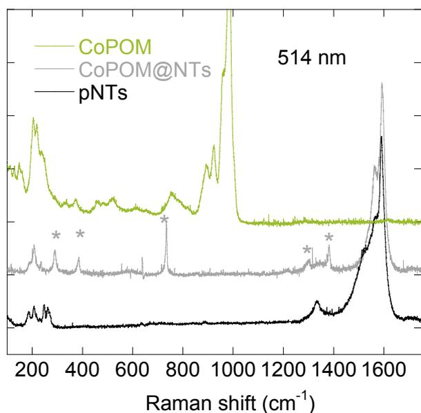
Figure S5 : Raman spectra of the pNTs, CoPOM@NTs and CoPOM molecule recorded under irradiation at 514 nm. The stars indicate resonances from the filter used as a support.
