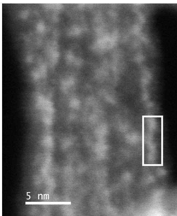
Figure S2: HAADF-STEM image of CoPOM@NTs at high magnification (scale bar: 5 nm) and inset area corresponding to the EELS spectrum displayed in Fig. 3.
