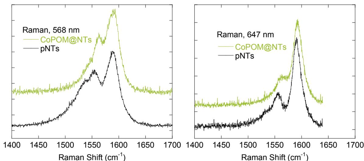
Figure S6 : Resonant Raman spectra focused on the G-mode area of pNTs and CoPOM@NTs under irradiation at 568 and 647 nm.
