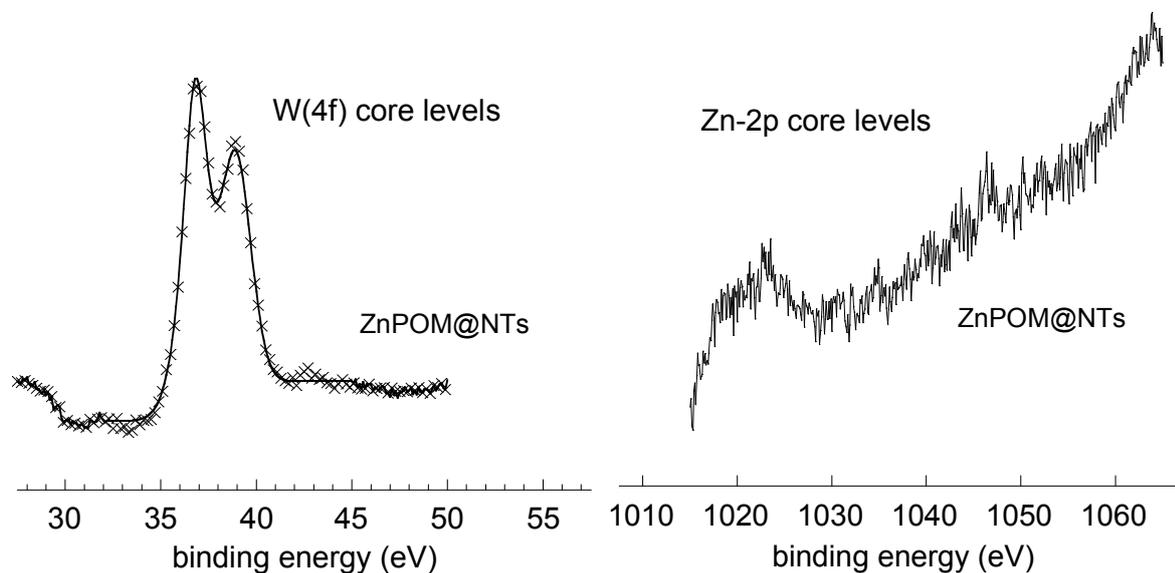
Figure S3: XPS spectra of ZnPOM@NTs focused on the W(4f) and Zn(2p) core levels.
