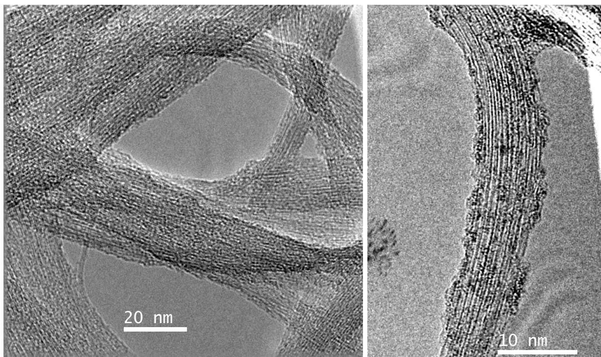
Figure S1: TEM image of pNTs (left, scale bar: 20 nm) and HRTEM image of CoPOM@NTs (right, scale bar: 10 nm)
