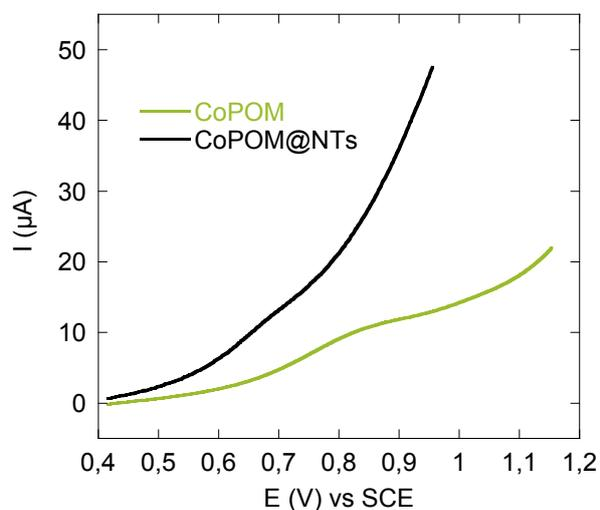
Figure S4: Voltammograms restricted to the Co-electroactivity domain of CoPOM@NTs-modified electrode and CoPOM deposited on a glassy carbon electrode. The reference electrode was a KCl saturated calomel electrode (SCE) and the counterelectrode a platinum gauze of large surface area. The scan rate was  $10 \text{ mV s}^{-1}$ .
