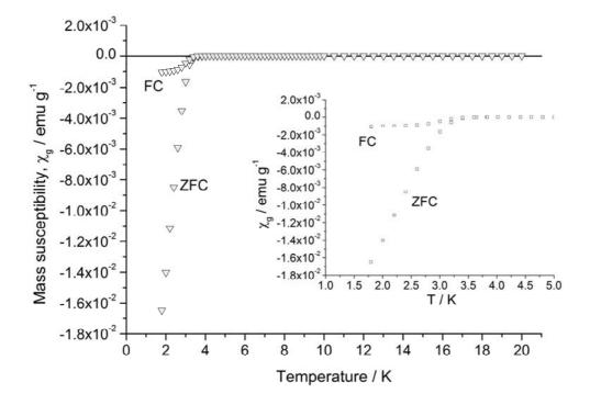
Figure S1 Plot of mass susceptibility vs. temperature for nanowires of 2H-TaS<sub>2</sub> (3).
