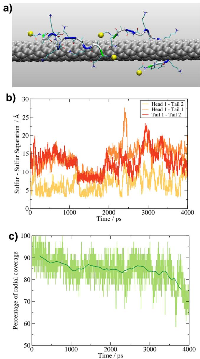
**Figure S3:** Evidence of formation of a 3-sulfur two-chain complex for the RC5/0.45 nm system. **(a)** Snapshot, with sulfur atoms indicated as yellow spheres. **(b)** Sulfur-sulfur contacts as a function of time. **(c)** Percentage of radial coverage as a function of time. The dark line indicates the running average of this coverage.
