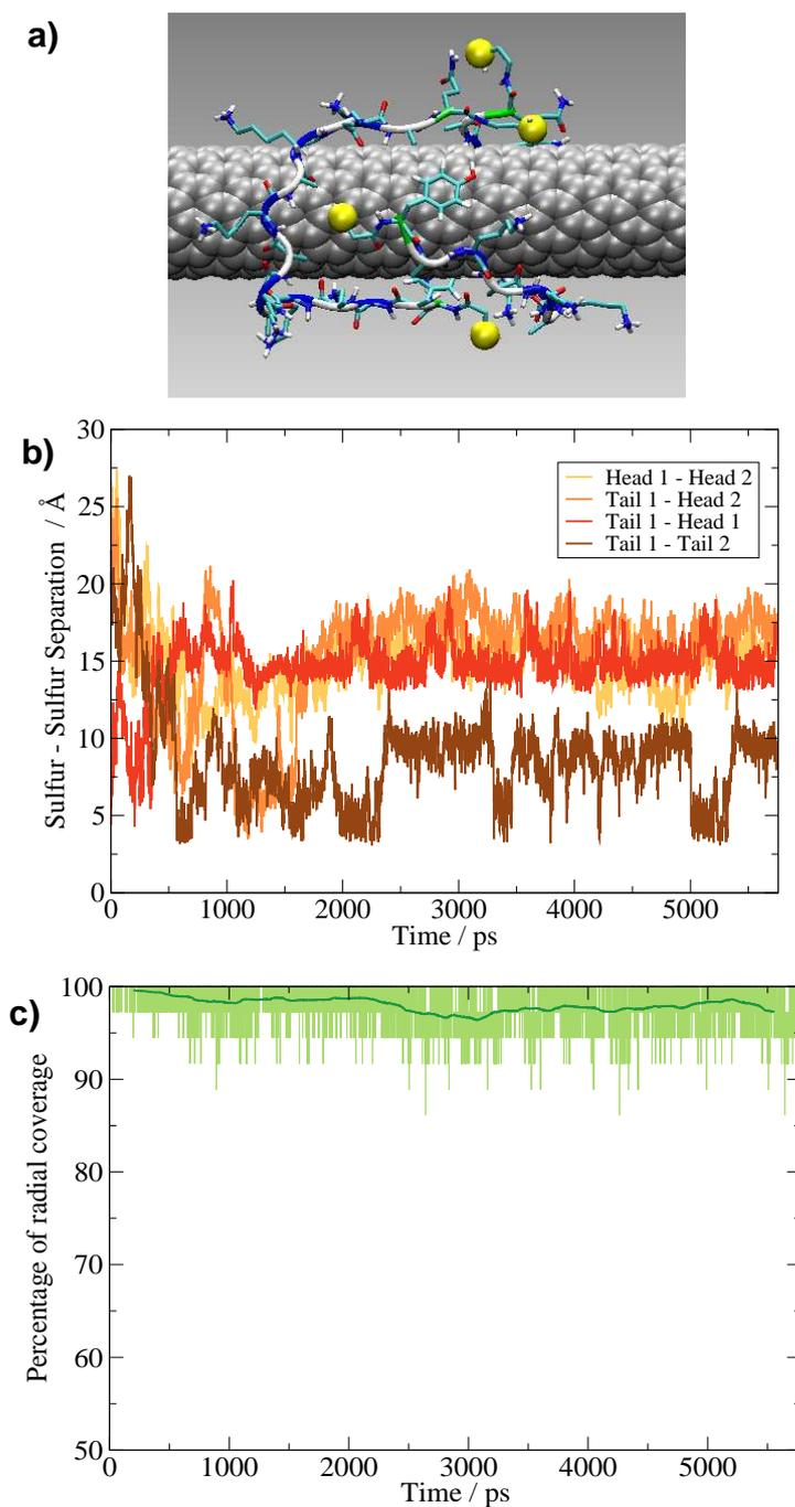
**Figure S7:** Evidence of a two interpenetrating half-wrap geometries for the RC7/0.75 nm system starting from a two side-by-side cyclised-wrap configurations. **(a)** Snapshot of final conformation, with sulfur atoms indicated as yellow spheres. **(b)** Sulfur-sulfur contacts as a function of time. **(c)** Percentage of radial coverage as a function of time. The dark line indicates the running average of this coverage.
