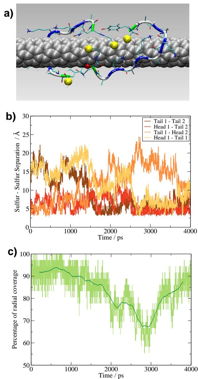
**Figure S2:** Evidence of formation of an interpenetrating half-wrap two-chain complex for the RC5/0.45 nm system. **(a)** Snapshot, with sulfur atoms indicated as yellow spheres. **(b)** Sulfur-sulfur non-bonded contacts as a function of time. **(c)** Percentage of radial coverage as a function of time. The dark line indicates the running average of this coverage.
