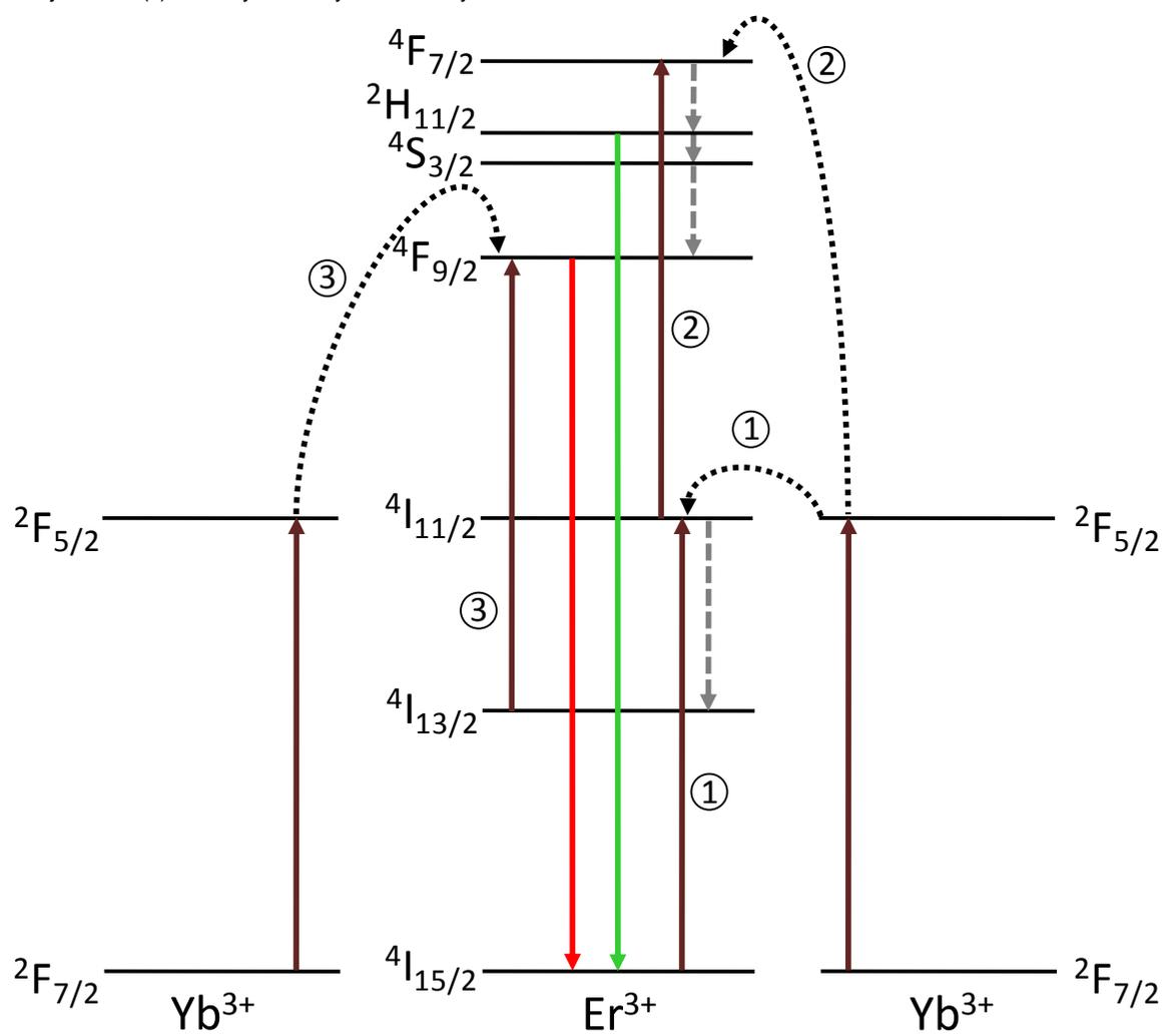
Figure S1: Schematic representation of the possible energy transfer processes involved in the upconversion of  $\text{Er}^{3+}/\text{Yb}^{3+}$  co-doped nanoparticles.
