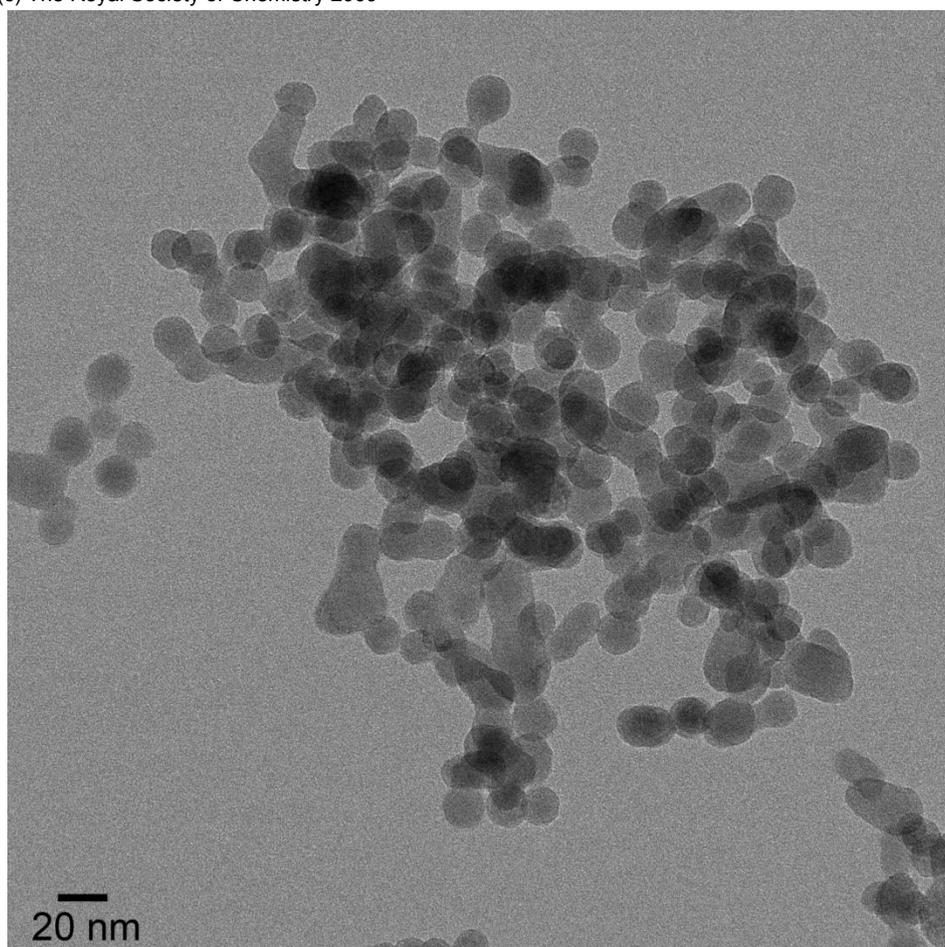
Figure S2: TEM image of the polyethyleneimine (PEI)-capped  $\text{NaYF}_4:\text{Er}^{3+}, \text{Yb}^{3+}$  nanoparticles.
