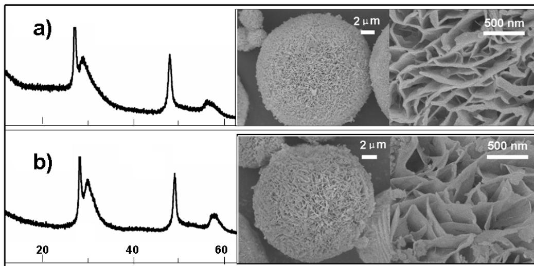
Figure S1. The XRD pattern (left) and SEM image (right) of ZnS microspheres a) before b) after the neutralization of the excess surface OH<sup>-</sup> by adding dilute acetic acid solution ( $1.0 \times 10^{-2}$  M ).
