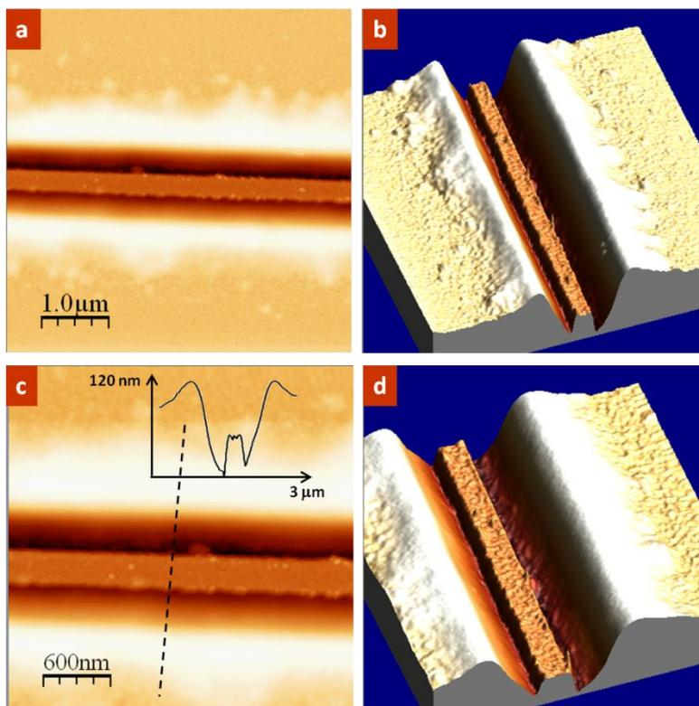
**Fig. 2S.** a) AFM image of the nanowire with the self-aligned trench after selective dissolution. b) 3D rendition of a). c) Magnified AFM scan of a). The inset is the height profile of the dotted line across the trench to show the sloped sidewall. d) 3D rendition of c).
