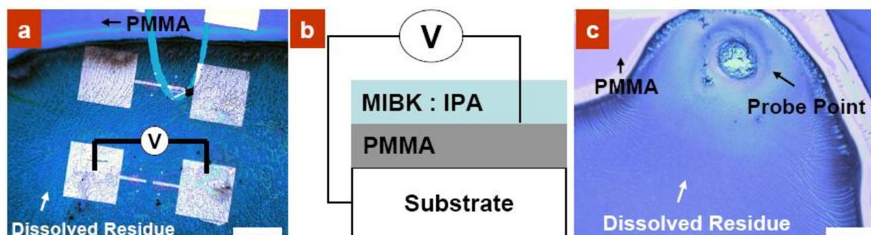
**Fig. 1S.** a) Optical image of PMMA dissolved in MIBK:IPA (1:3) in the presence of an electric field; b) Schematic of electric-field induced dissolution experiment; c) Optical image of PMMA pattern obtained. Large area dissolution occurred within a short time (100 s). Scale bar: 400  $\mu\text{m}$ .
