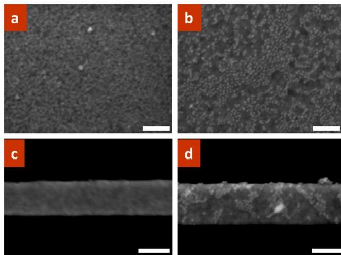
**Fig. 3S.** SEM images of gold surfaces without DNA modification (a, c) and with capture DNA strands (b, d) after gold nanoparticle assembly, respectively. Scale bars: 200 nm.
