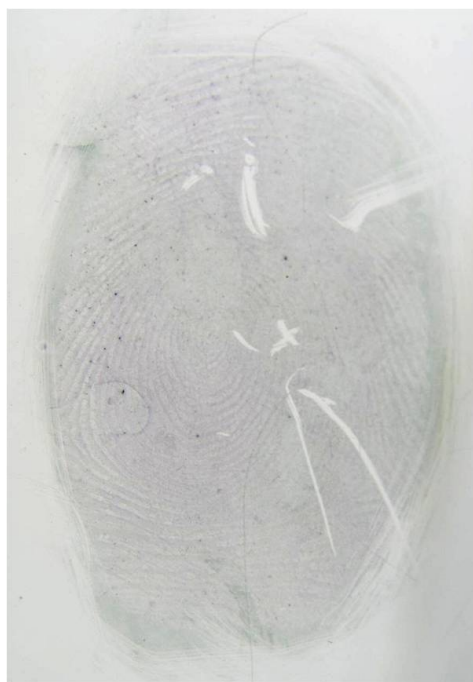
Figure S2. Optical image of latent fingerprints after development by in-situ growth of gold nanoparticles on ridge patterns on a plastic Petri dish.
