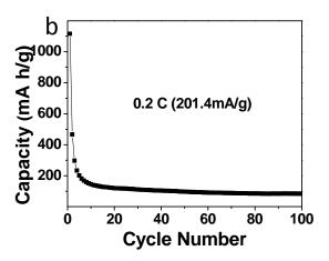
Figure S1 (a) FESEM image of the pure  $Fe_2O_3$  nanoparticles and (b) charge/discharge cycling performance of the  $Fe_2O_3$  electrode at current densities of 201.4 mA/g (0.2 C) within a voltage window of 0.01-3.0 V.
