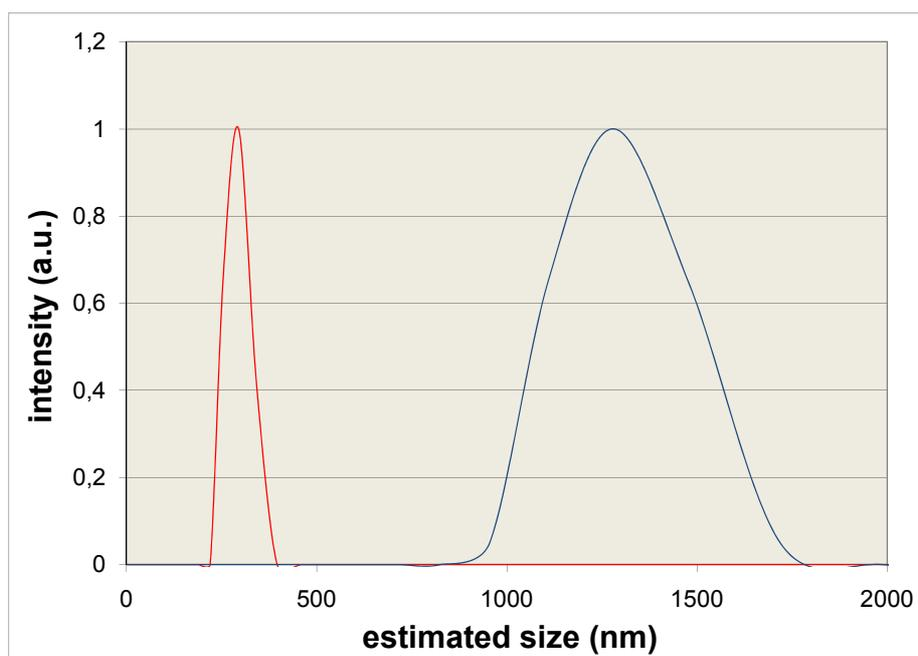
**Figure S1.** DLS diagrams of *ox*-SWCNTs **1** in PSF (top) and HRP (bottom) at time zero (blue line) and after 60 days (red line).
