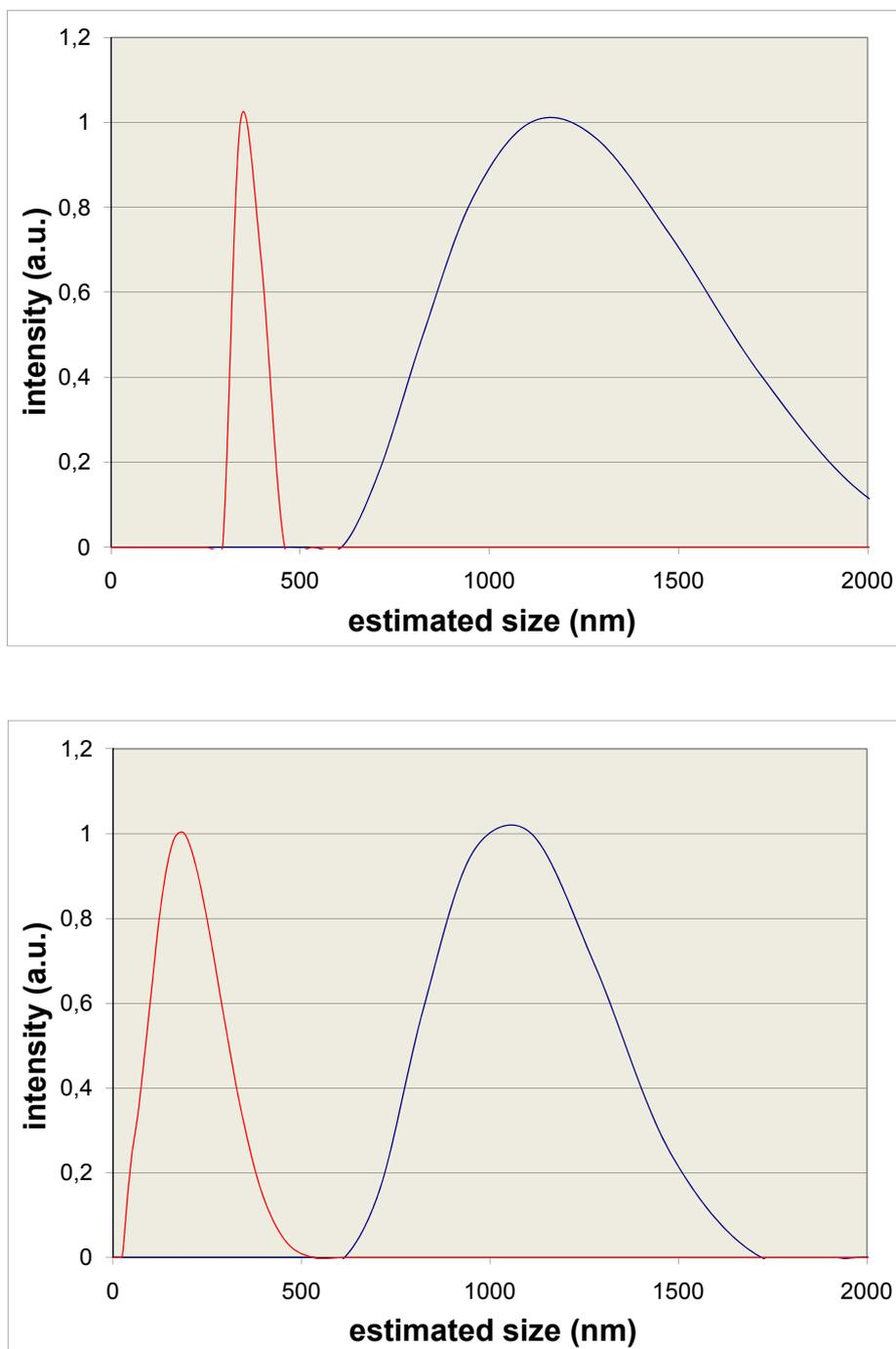
**Figure S3.** DLS diagrams of  $\alpha$ -MWCNTs 3 in PSF (top) and HRP (bottom) at time zero (blue line) and after 60 days (red line).
