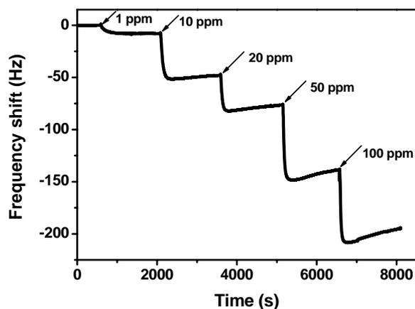
Fig. S1. Response during exposure to increasing TMA concentrations of PAA/NaCl (0.1 wt%) CNMs coated sensor with a coating load of 1100 Hz.
