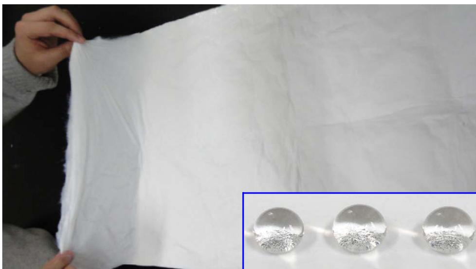
Fig. S1 Several water droplets placed on the PS fibrous mats formed from DMF with 7.7 wt% silica showing the superhydrophobicity.
