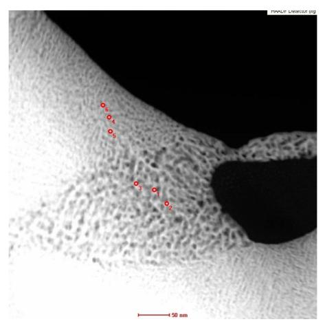
Fig. S2. HAADF-STEM image showing the microstructure of the np- $Pt_{60}Au_{40}$  NCs fabricated by dealloying the rapidly solidified  $Al_{75}Pt_{15}Au_{10}$  precursor in the 20 wt.% NaOH solution. The positions for NB-EDX analysis are highlighted by small circles with the numbers 1-6 beside.
