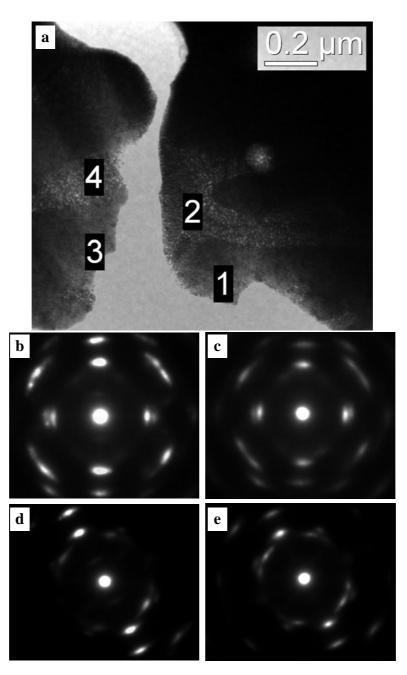
Fig. S1. (a) TEM image showing the microstructure of the  $np-Pt_{60}Au_{40}$  NCs fabricated by dealloying the rapidly solidified  $Al_{75}Pt_{15}Au_{10}$  precursor in the 20 wt.% NaOH solution, and (b-d) SAED patterns corresponding to the positions 1-4, respectively.
