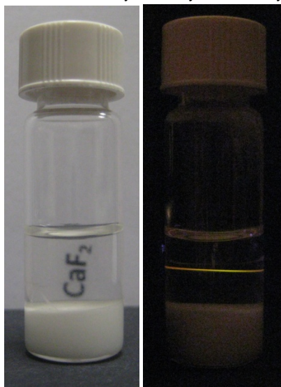
Figure S6. Extraction of the \text{CaF}_2 nanoparticles from a \text{CHCl}_3 dispersion (lower layer) to a sodium oleate aqueous solution (upper layer). The aqueous solution is perfectly transparent (left image) and the UC emission is very bright upon laser excitation at 980 nm (right image). The lower layer is milky due to a partial transfer of the oleate molecule into the \text{CHCl}_3 dispersion.
