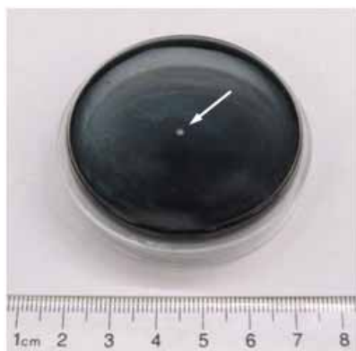
Figure S5. Photograph showing the white spot, indicated by the white arrow, on the bottom surface of the petri dish after HIFU irradiation at a power of 15 W for 5 seconds.
