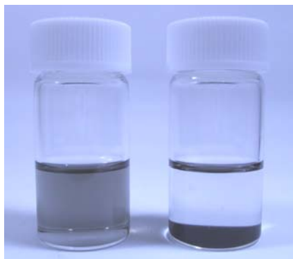
Fig. S1 Photograph of NMP solutions of the SWNTs before (left) and after (right) the addition of the NH 2 -silica.
